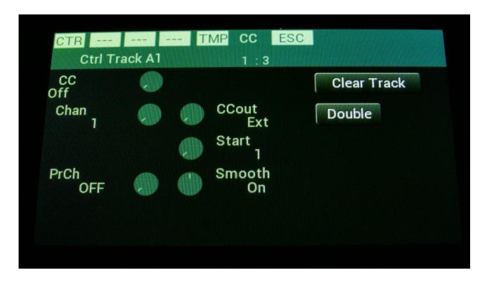
The CC parameter can be set to any MIDI CC between 1 and 126. In the top position, you will find Pitch Bend, and at position 16 (CC16), you will find the touch screen keyboard Y-position.
