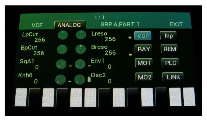
Adjusting the Cut and Reso parameters on the VCF page, when the filter is in Frame Sequencer mode, will set an offset for these parameters, affecting all filter frames at the same time.
