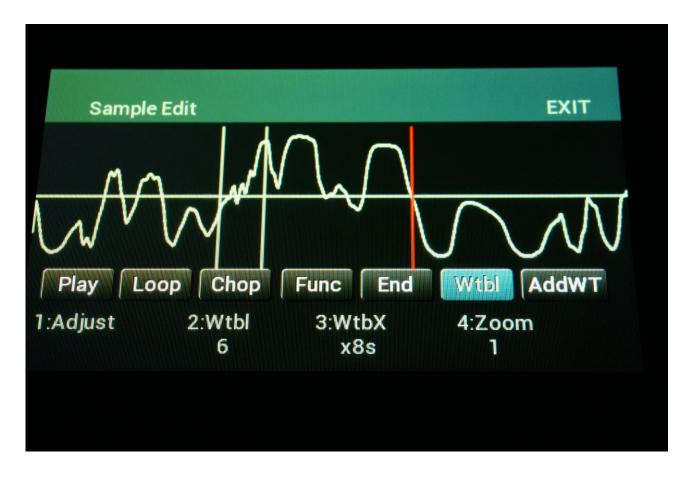
On the graphical sample edit page, with the sample, which you would like to build a wavetable from, selected, touch the Wtbl button, so that this turns blue. Zaturn will now create one wave for a table, consisting of 512 sample points, equally spaced between the selected start and end points. As soon as Wtbl mode is switched on, the currently generated wave will be audible.
