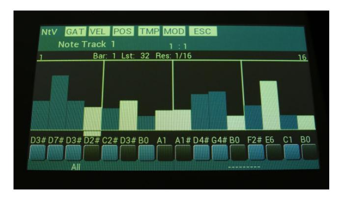
You can now, by turning Edit Knob 1, adjust the offset of all steps at the same time. Middle position of Edit Knob 1 is zero, above middle will turn the offset up, below middle will turn the offset down.
