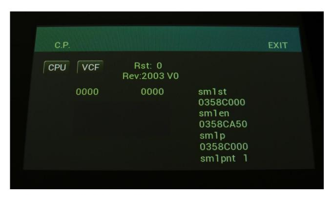
This is a service page, and does not really have any practical user functionality, except for the "CPU" touch button. If you touch this, so that it turns blue, Zaturn will show how much CPU power is used, on the Preset Select page.
