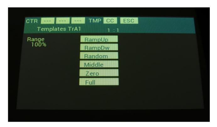
First turn Edit Knob 1, to set the range. This will set, how much the template routine will affect the values, that are already on the selected subtrack. When this is set to 100%, the template function will be absolute. Then touch any of the template boxes in the right side of the screen.
