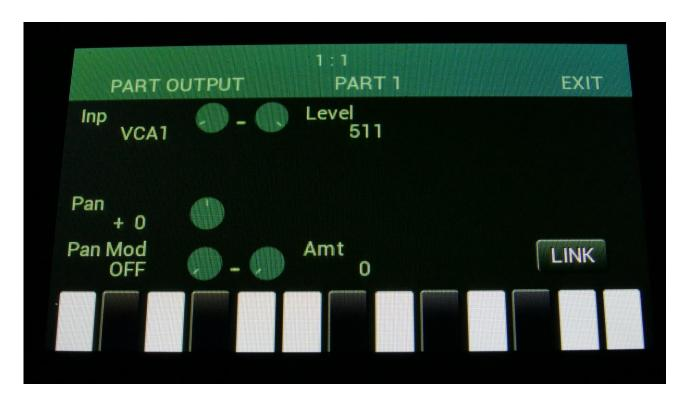
Select the output module for the desired part, by pushing and holding the Steps/Part button, while pushing one of the 8 trigger buttons.
