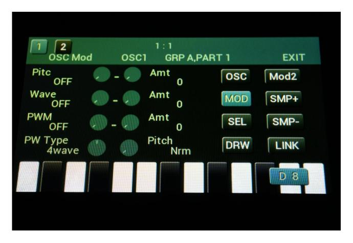
For each parameter, that can be modulated, it is possible to select a modulation source and to adjust the modulation amount. For a complete list of modulation sources, see the "Connecting Modules" chapter.
