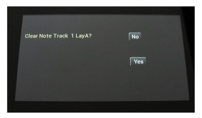
Touching "Yes" from here, will initialize all step values and parameters on the selected Morph Layer of the currently selected note track, except for the Last Step parameter. Select the Morph Layer with the Morph function button.
