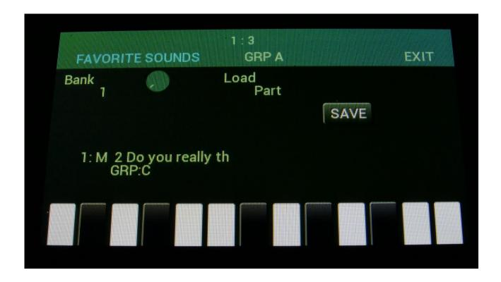
When on the favorite sounds page, pushing a step button will load a sound to the currently selected Group, while playing the sound back for auditioning, and showing the preset and group location on the display. Step buttons that has a favorite sound stored, will light up.
