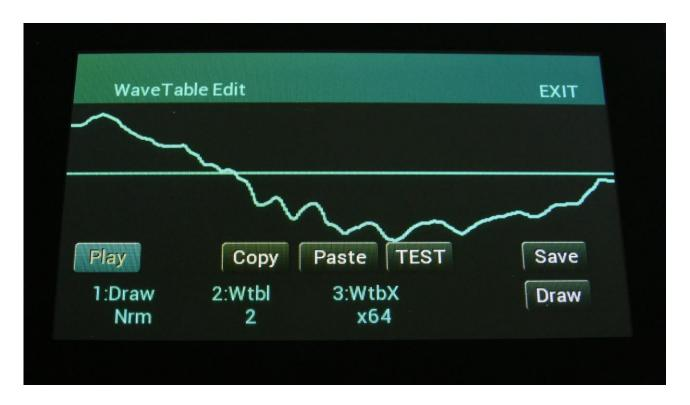
You can keep this turned on, while you are drawing. The output sound will change, according to the wave.
