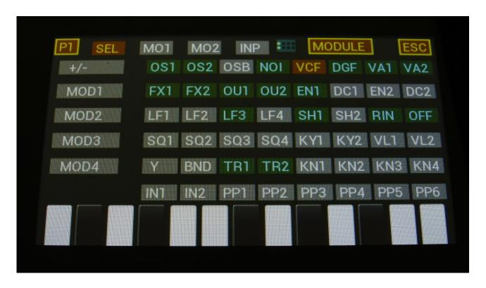
To connect modules on the overview page, first touch the SEL button in the top of this page. The SEL button should now turn brown. Then touch the module, for which you want to connect the modulation/inputs. This module will now turn brown. Then touch either the MO1 (modulation page 1), MO2 (modulation page 2) or INP (audio inputs) in the top of this page, depending on what you wish to connect.
