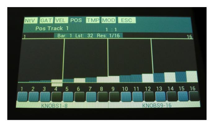
Unlike many other step sequencers, the position for each step on the Zaturn note tracks, can be set. For traditional step sequencing, you would leave it at its default setting, when step 1 is played back at position 1, step 2 is played back at position 2 and so on.
