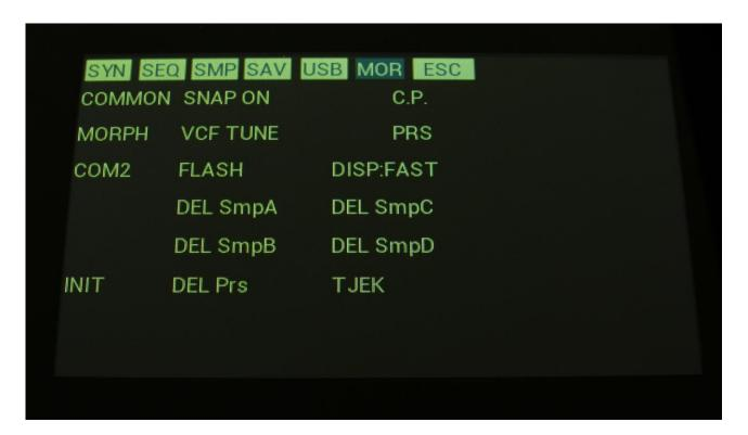
On the MOR page, touch the "SNAP OFF" text. The text will now change to "SNAP ON", and the parameter snap feature will be turned on.
