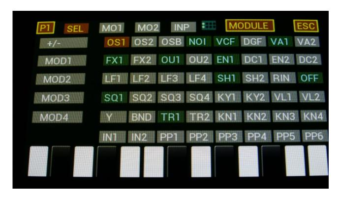
On this page you have an overview of all the synth modules of one module group, and you can easily see which modules are used by the currently selected part. The colored modules are used by the part, the grey modules are not. You can select parts 1-8, by pushing and holding the Steps/Part button, while pushing a step button.
