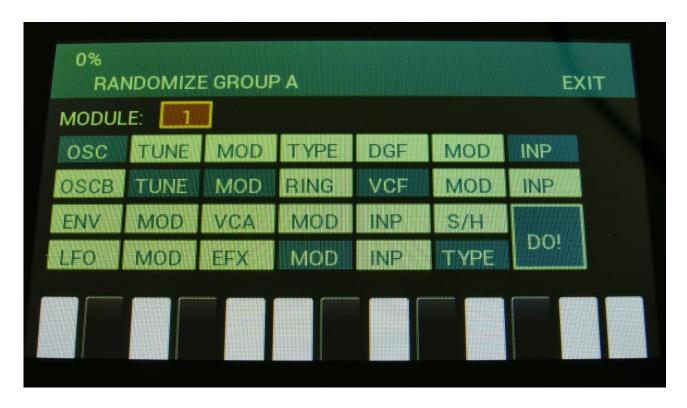
First, make sure that you have selected the right group, in which you want to randomize the parameter values. You can do that, by pushing and holding the Steps/Part button, while pressing one of the 8 step buttons. The selected group is shown at the top of this page.
