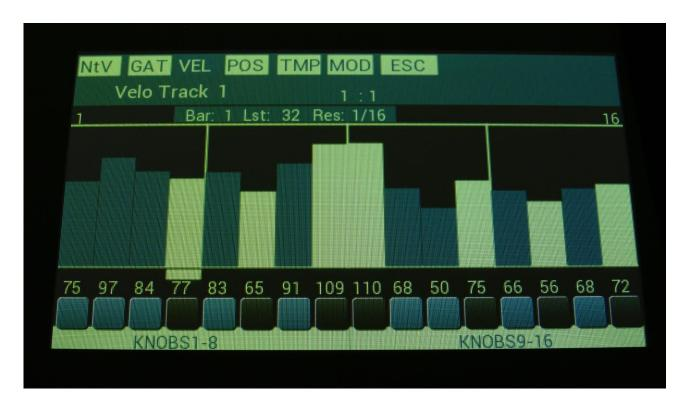
The velocity values for each step is shown as bars in the value grid, and as number right below the value grid. Velocity values for each step can be changed, simply by touching the value grid. Values can also be changed, using edit knob 1 to 8. In the bottom of the page, touch the field named "Knobs 1-8", to edit the first 8 steps, using the edit knobs, or touch the field named "Knobs 9-16", to edit the last 8 steps, using edit knob 1 to 8.
