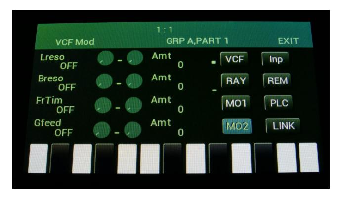
On the VCF MO2 page, you will find the FrTim parameter. Setting this up to a modulation source, and turning up the amount, will make it modulate the frame transition times.
