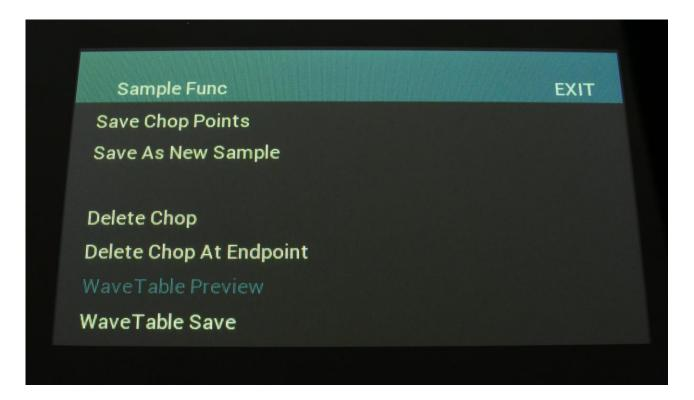
Touch **WaveTable Preview**, so that this turns blue. Now you will hear your wavetable playing back. Adjust **Edit Knobs 1** and **2**, to scan through the waves (**Edit Knob 2** is only active at 64 waves).
