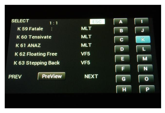
Touch "PREV" or "NEXT" to view the previous or next 5 presets, touch the buttons named A to P to select a specific preset bank, and finally touch the preset name of the preset you would like to select. 1024 presets can be selected, from A01 to P64.
