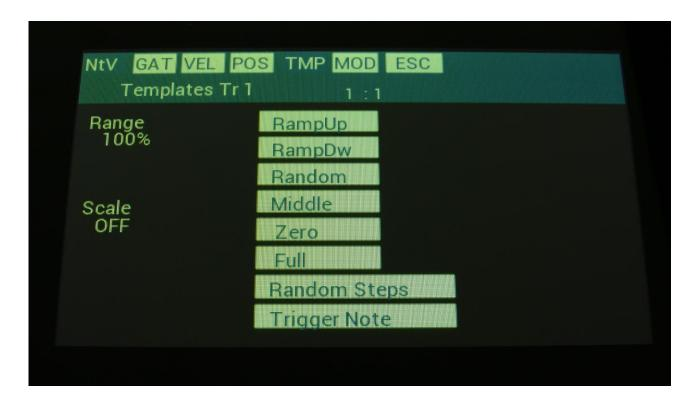
First turn Edit Knob 1, to set the range. This will set, how much the template routine will affect the values, that are already on the selected subtrack. When this is set to 100%, the template function will be absolute. Then touch any of the template boxes in the middle of the screen.
