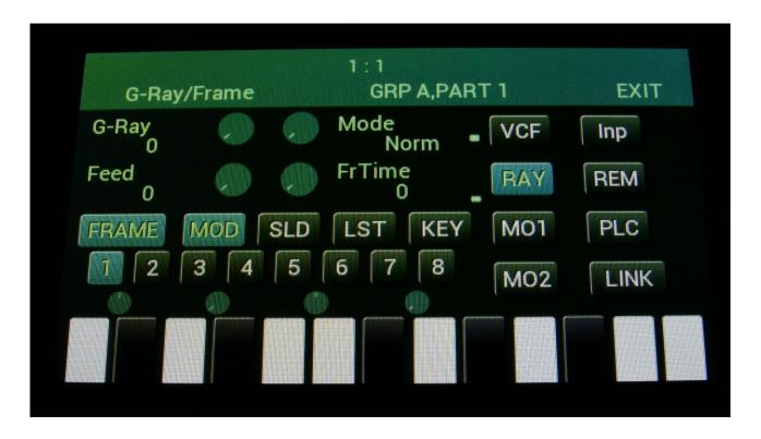
To make even more advanced filter frame sequences, it is also possible to include the G-Ray Feed, Outp, and all modulation amount parameters in each frame. To do so, hit the **MOD** button, so that it turns blue.
