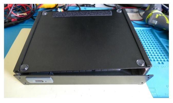
Flip your zaTurn around, so that the bottom is facing upwards.
