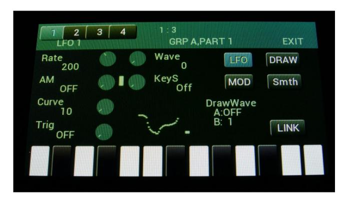
Each group has 4 LFO's (16 in total) with a waveform that morphs from triangle to sawtooth to pulse to FM waves. Curve can be morphed from logarithmic over linear to exponential. In the S-Shape modes, the LFO's will morph from logarithmic S-shape over logarithmic to linear to exponential to exponential S-shape.
