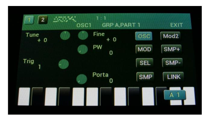
In the upper left corner of the oscillator page, the currently generated waveform is shown.
