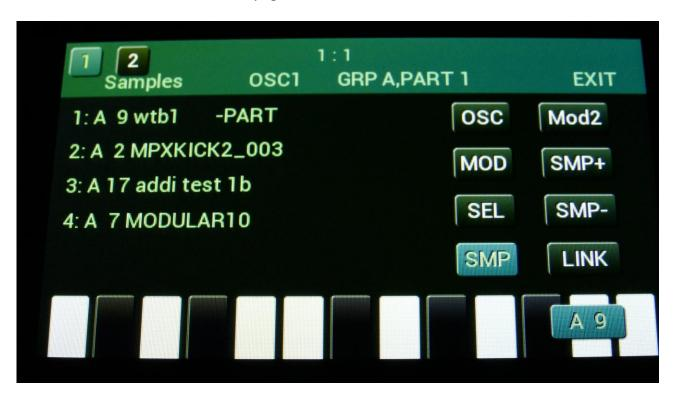
Here you can select 4 samplings for the part. The number of these samplings, that are used, is set by the #Smp parameter on the SEL page. The 4 samples can be selected to play back, setting the Chop parameter, and by chop select modulation.
