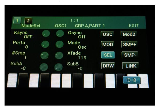
**Ksync:** Key Sync (Oscillators only). Can be set to off, or to a specific amount between 1 and 511, which indicates the start point of the oscillator waveform, that is the point at where the waveform generation will start, every time the oscillator is trigged from the part trigger.
