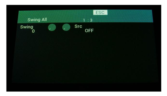
Swing All will let you add modulated swing to all 8 note tracks at the same time. For creating traditional swing, you should modulate with a controller track, and program the swing pattern on this, but on Zaturn, any modulation source can be used for swing, so there are quite a lot of possibilities to deform a sequence with this.
