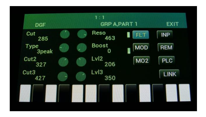
The 4 digital filters on Zaturn have 28 different filter types to choose from. Cutoff frequencies, resonance, triple filter levels and formant morphs\* can be adjusted and modulated.
