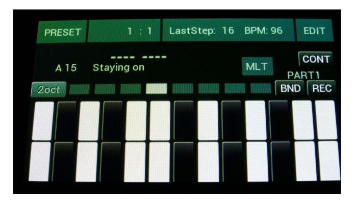
To change the number of touch keyboard octaves, touch the "oct" switch, which is located to the left, right above the keyboard. Every time you touch it, it will toggle between 1oct, 2oct and 3oct. When 2 octaves are selected, the upper and lower octaves get divided by a line in the middle of the keyboard. When 3 octaves are selected, the upper, middle and lower octaves get divided by 2 lines.
