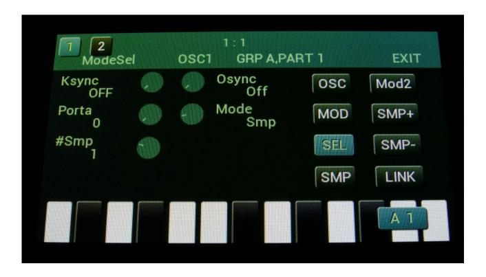
Set the Oscillator in sampler mode, and touch the SMP touch button to select the sampling, that you just wave chopped (or any other sampling that you have wave chopped).
