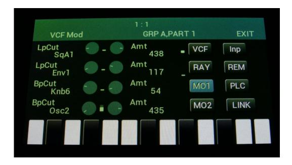
The "manual" way, is to go to a modules audio or modulation input pages, select the audio/modulation source, using Edit Knob 1 to 4, and adjust the amount/level, using Edit knob 5 to 8. Only positive sources can be selected this way.
