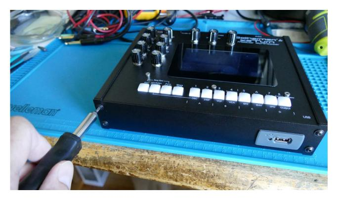
Turn zaTurn over and mount the hex screws. You will need to hold the end panel in place, when you are mounting these screws.
