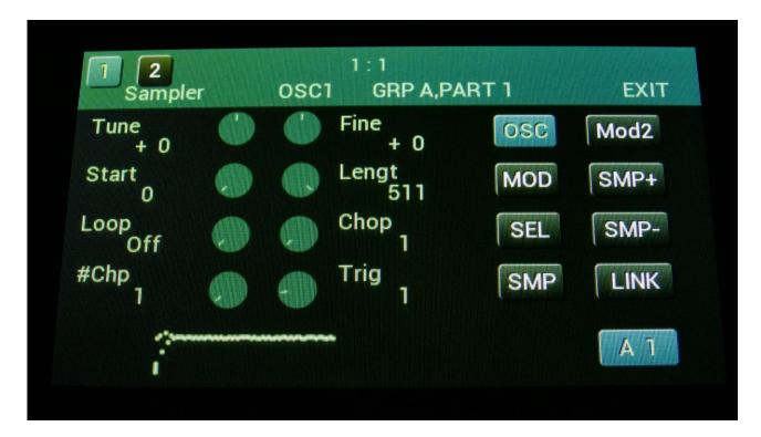
In the bottom of the sampler page, the selected samplings waveform is shown in rough graphics. When the sample, or part of it, is played back, the small white line below the waveform will show the current playback point.
