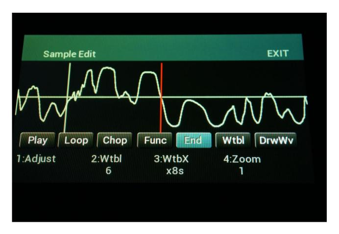
By touching the End touch button, so that it turns blue, the screen will now be focused on the end point, which is indicated as a vertical red line. When you touch the screen now, the red line will move, indicating that the end point is selected. It is also possible to change the end point, by rotating Edit Knob 1.
