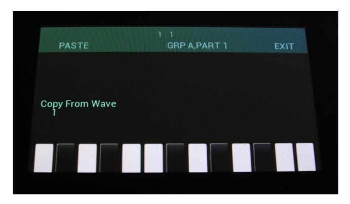
When pasting LFO's or Oscillators which uses draw waves, these are automatically pasted together with the LFO/Oscillator parameters.
