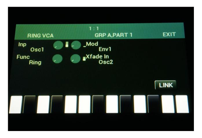
Each group has one Ring VCA (4 in total), which can be used as both VCA's, Ring Modulators, CrossFaders, as logic modules and as mixers.
