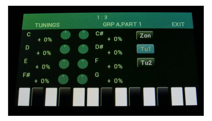
Here it is possible to microtune each note in an octave by up to +/- 50 percent. This is possible separately for each of the 8 parts, but it is only possible for the Type2 and Resonator oscillators. The Type1 oscillators, the samplers and the noise generators are not affected by these settings.
