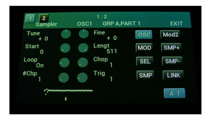
Set Loop mode to On, and adjust the Chop parameter, to select the single cycle waves. If you would like more single cycle waves to play back inside the loop, turn the #Chp parameter up.
