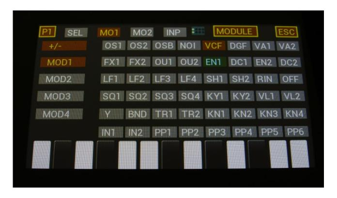
If you, for instance, touched MO1, MOD1 in the left side of the page will now also be selected, and the module which turn green, is the module which is connected to the MOD1 (modulation source 1) of the MO1 page.
