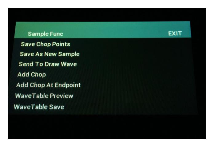
Touch "Save As New Sample". A new page will now open. Select the sample bank, that you would like to copy the sampling/portion of the sampling to, by touching the A, B, C or D touch button.
