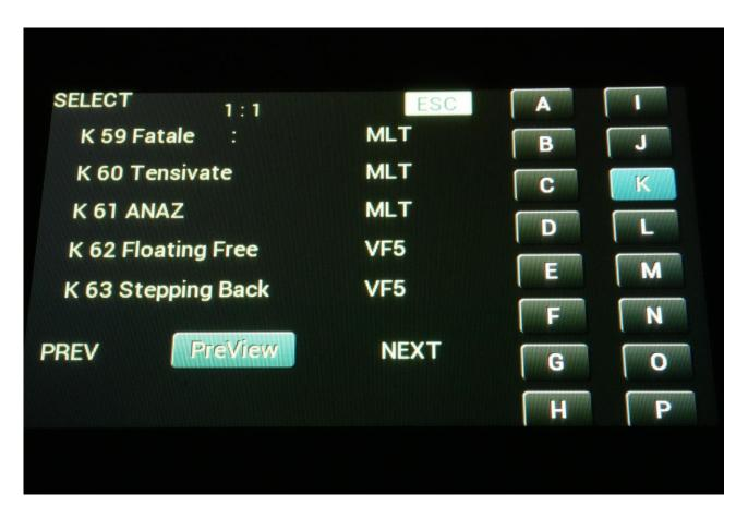
If the sequencer is running, it will still wait for track 1 to reach step 1, until it jumps to the next preset. This is indicated by the Play LED flashing. Here it is also possible to make the preset switch happen immediately, by pushing the Play button, while it is flashing.
