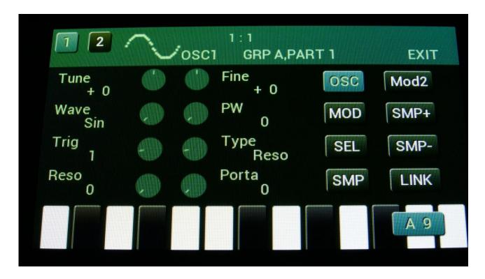
Touch the buttons named OSC, MOD, SEL, SMP and Mod2, to enter other oscillator pages, like Modulation and oscillator/sampler/noise/Wavetable mode select.
