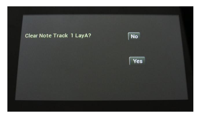
Touching "Yes" from here, will initialize all step values and parameters of the currently selected note track, on the currently selected Morph Layer (Morph function button selects the layer), except for the Last Step parameter.
