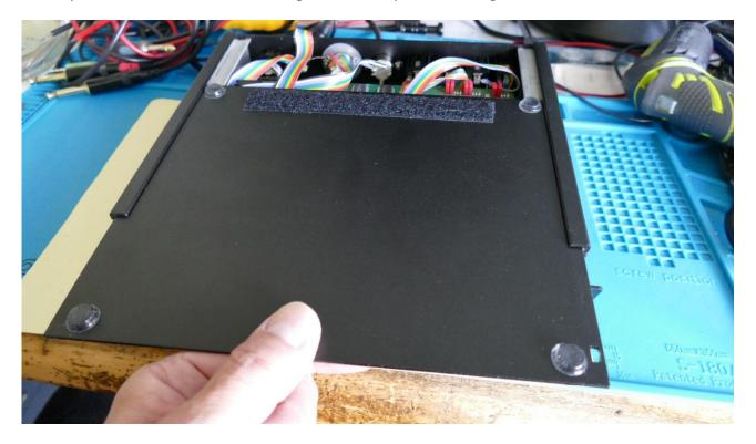
Slide the bottom panel back in to place. Take care, that all cables are inside, and that they are not "ran over" by the panel.
