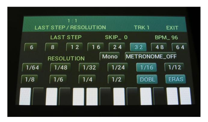
**Setting the tempo:** Turn Edit Knob 4 to set the tempo for the current sequence. The tempo is shown in BPM's (beats per minute) in the upper right corner of this page, and can be set between 51 and 306 BPM's.
