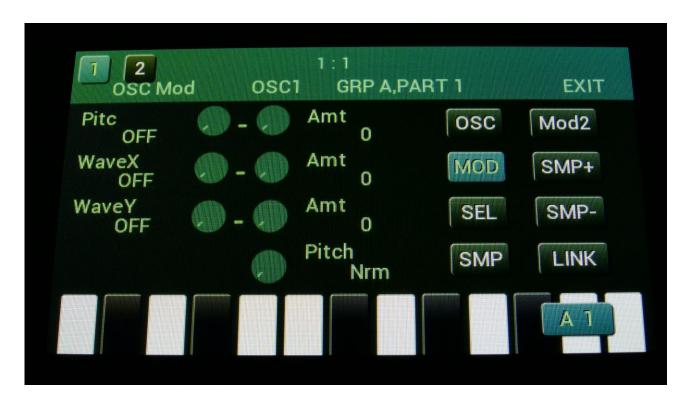
For each parameter, that can be modulated, it is possible to select a modulation source and to adjust the modulation amount. For a complete list of modulation sources, see the "Connecting Modules" chapter.
