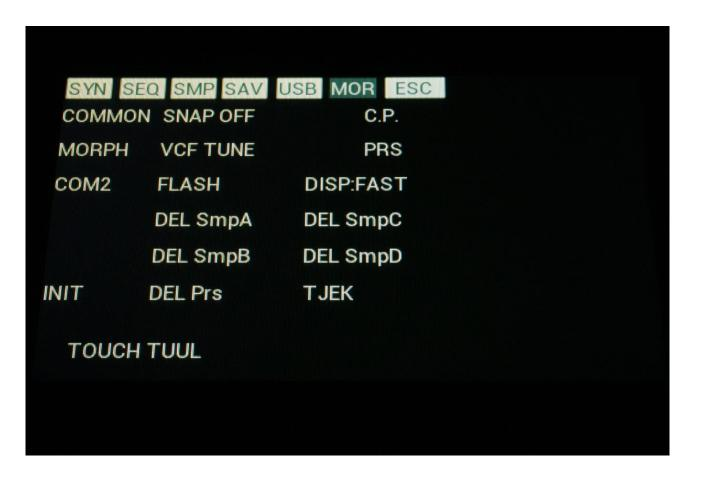
This will get you to the MOR page. Here you can set up all the basic Zaturn things, like global MIDI channel, morphing, tune the analog filters, check and erase the Zaturn memory, initialize the preset and change to song mode.
