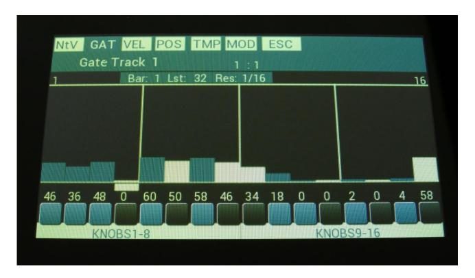
The gate time values for each step is shown as bars in the value grid, and as number right below the value grid. Gate time values for each step can be changed, simply by touching the value grid. Values can also be changed, using edit knob 1 to 8. In the bottom of the page, touch the field named "Knobs 1-8", to edit the first 8 steps, using the edit knobs, or touch the field named "Knobs 9-16", to edit the last 8 steps, using edit knob 1 to 8.
