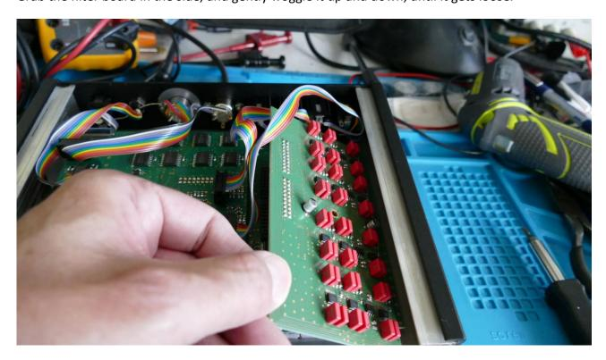
Lift the side of the filter board, which is pointing towards the middle of the casing, up a bit, and take the board out.
