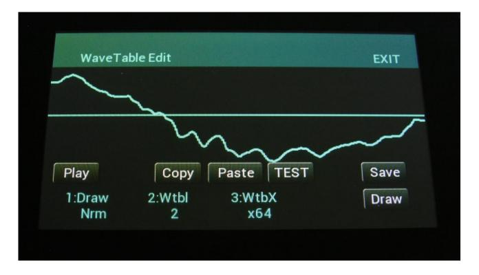
Here you can view and edit the wavetable one wave at a time. With **Edit Knob 2** you can select wave 1 to 8 or 1 to 64, depending on the wavetable mode. With **Edit Knob 3**, you can select the desired mode: **x8** (8 waves) or **x64** (64 waves) or **x8s** (8 serum waves).
