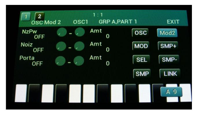
For each parameter, that can be modulated, it is possible to select a modulation source, either directly or by group (Func/Mute / Steps/Part held), and to adjust the modulation amount. For a complete list of modulation sources, and complete instructions, see the "Connecting Modules" chapter.
