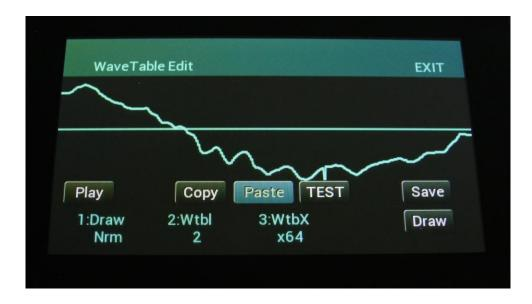
At any time under this process, it is also possible to test the wavetable. Touch the TEST button, so that this turns blue.
