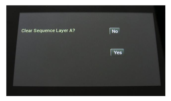
If you touch the "Yes" button here, Zaturn will clear all tracks on the selected Morph Layer (select Morph Layer with the Morph function button) of the current preset, and reset all values.
