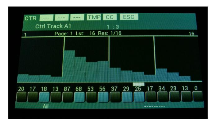
This will be the first page you will enter, showing the controller values, that will be outputted for each sequencer step, when the sequencer is playing back.
