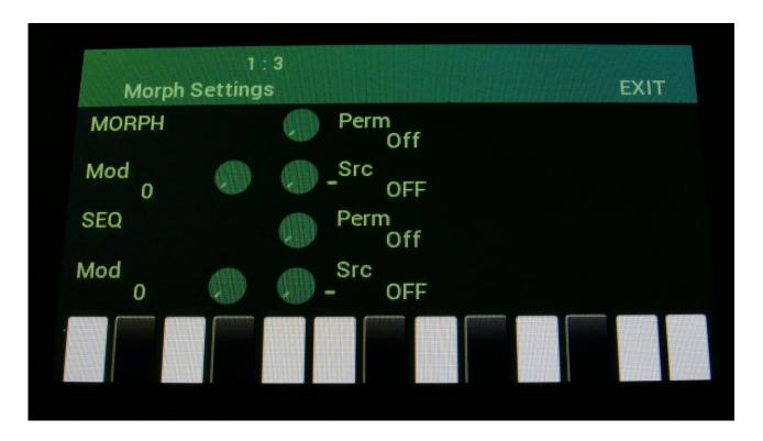
The upper row of parameters is the settings for the Morph knob, that affect the Synth Parts. The lower row of parameters is the settings for the Seq Morph knob, that affect the Sequencer tracks.
