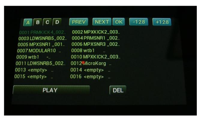
Touch A, B, C or D to select sample bank A, B, C and D, touch PREV and NEXT to view the previous or next 16 samplings. Touch the -128 and +128 buttons to skip 8 pages at a time.
