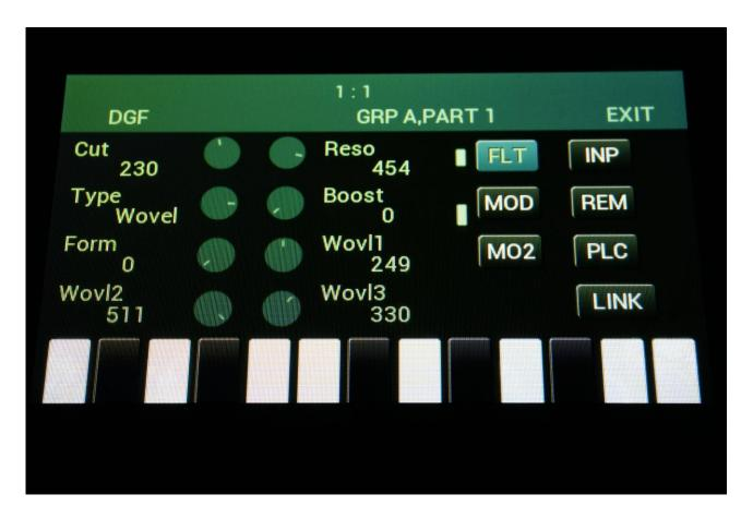
This filter is composed of three bandpass filters. 32 formants can be selected. Each formant has the cutoff frequencies and levels of each of the bandpass filters pre-programmed, to generate a wovel. Five formants can be selected at a time, using the **Wovl1 to 5** parameters, and it is possible to morph through these, using the **Form** parameter. The **Form** parameter can also be modulated by any modulation source, for automated morphing through the selected formants.
