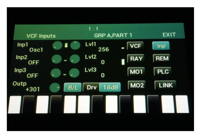
When this is switched on (blue), the filter input levels can be adjusted to get the desired amount of drive.
