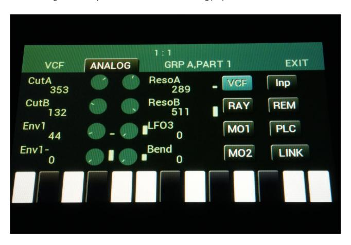
This filter board adds two analog filters to each Group (8 in total), based on the VCF2 filter board, but with some added features, like 24db filter modes and self-oscillating resonance.
