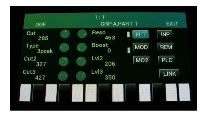
The 4 digital filters on Zaturn have 27 different filter types to choose from. Cutoff frequencies, resonance and triple filter levels can be adjusted and modulated.
