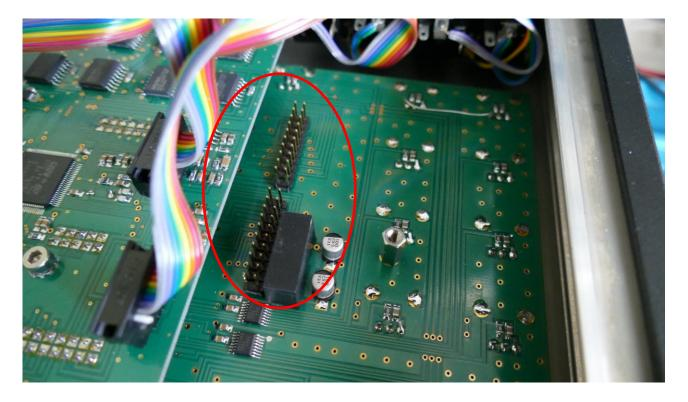
zaTurn without an analog filter board. Please notice the 2 connectors. You will now have to mangle the new filter board in, and connect it to these.
