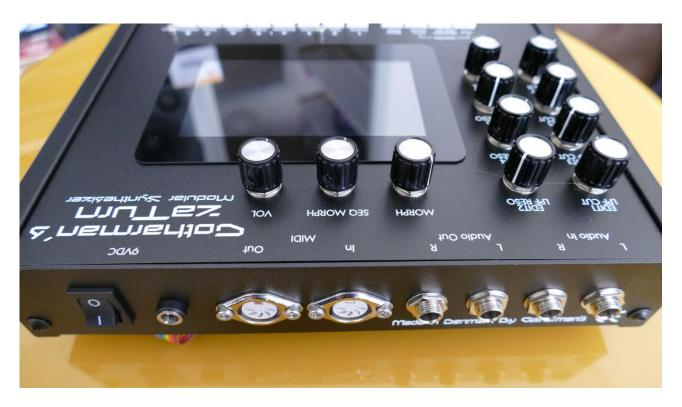
On the back panel of your Zaturn, you will find the power switch, connection for power supply, audio inputs and outputs and MIDI in and out.
