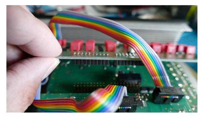
Before you push the filter board into place, inspect and make sure, that the connectors are perfectly aligned. Now push the board into place.
