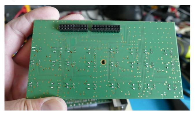
The back of the filter board also has 2 connectors.
