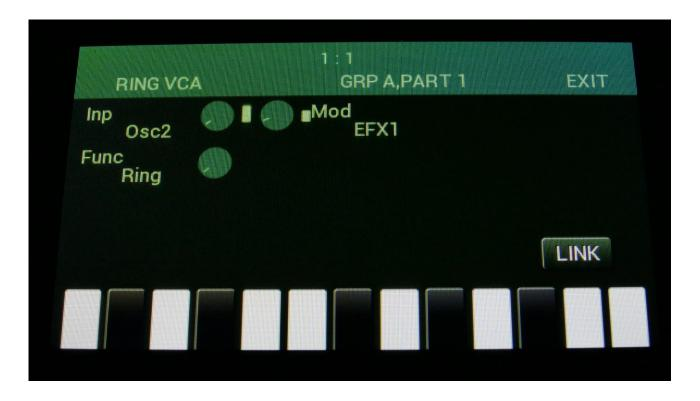
Each group has one Ring VCA (4 in total), which can be used as both VCA's, Ring Modulators, as logic modules and as mixers.
