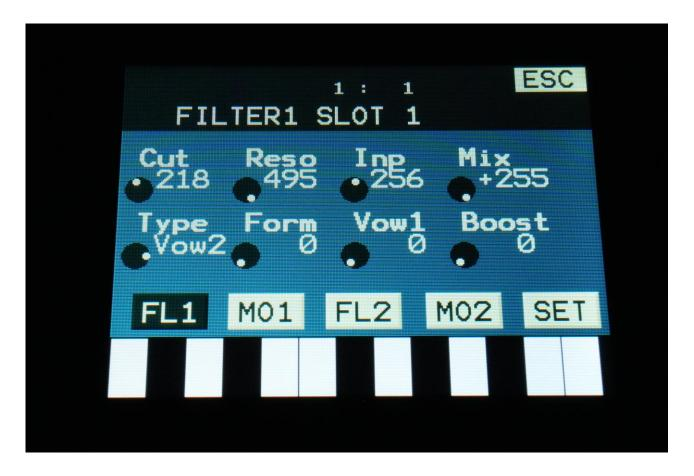
When one of the vowel filter types is selected, the following parameters are available on the FL1 page. On the Poly Touch model, these parameters are also available on the FL2 page.
