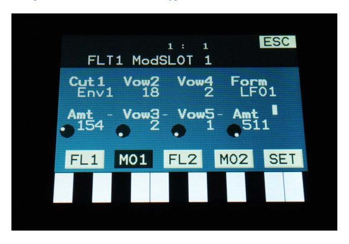
**Cut1:** Will modulate the filter cutoff frequency offset.
