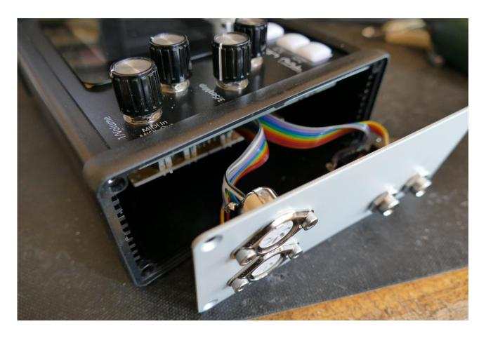
Mount the left end panel, and put the 4 screws back:
