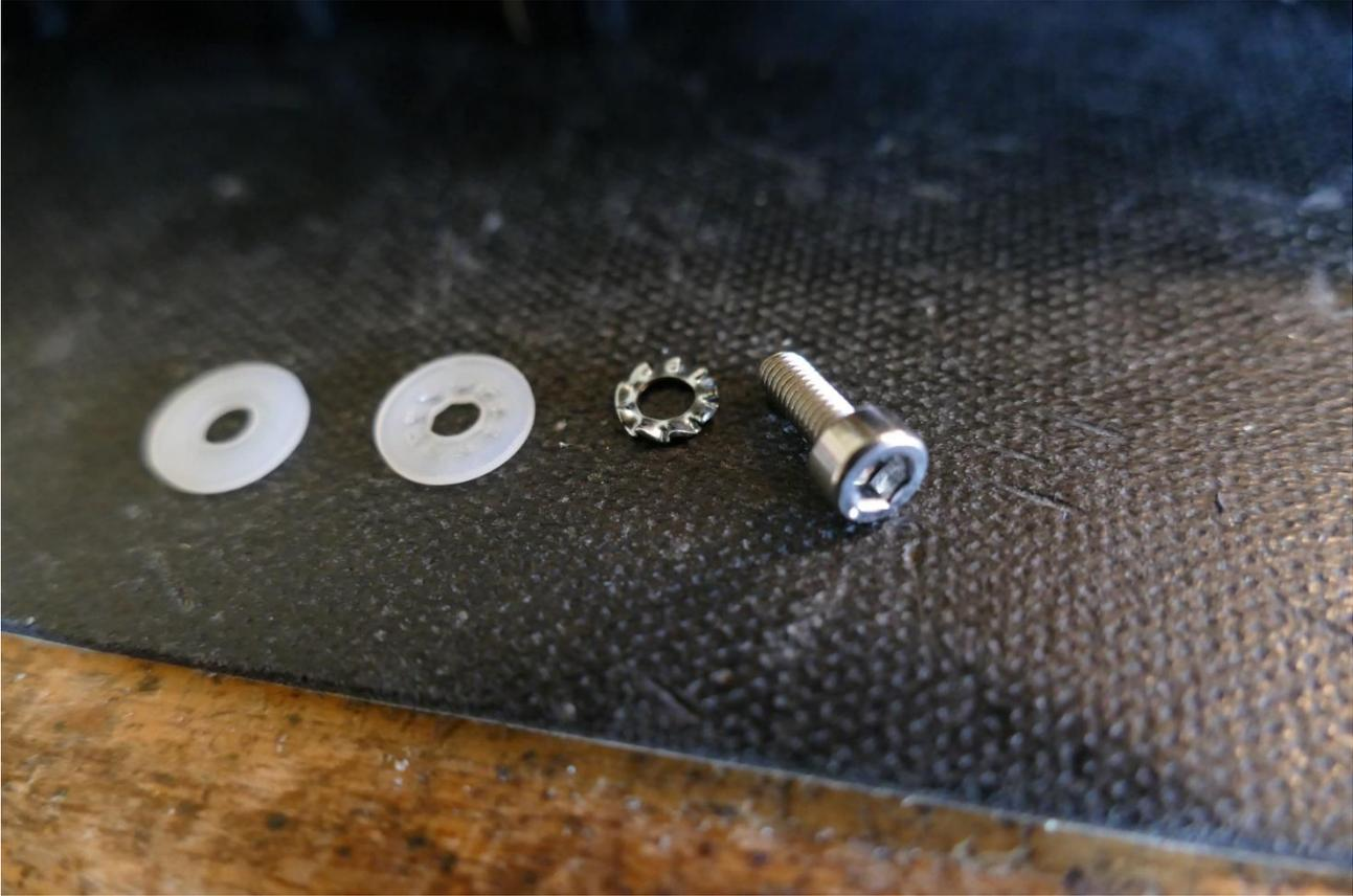
Before you start installing the new filterboard, you should assemble the screw and the washers like this:
