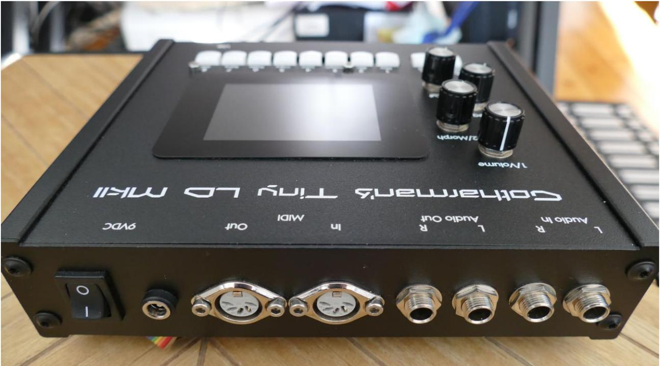
On the rear panel of your Tiny LD MkII, you will find the power switch, connection for power supply, MIDI in and out, and stereo audio inputs and outputs.
