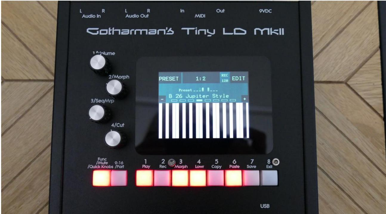
Tiny LD has a highly sensitive and responsive capacitive touch display, 8 step/trigger/part select/function buttons, a Func/Mute button, and a Steps/Parts 9-16 select/Part Select button. It has 4 Edit Knobs for controlling and editing parameters and sending MIDI CC's, that doubles as Volume, Morph and sequencer Morph knobs. Only Edit Knob 4/Cut are assignable, to control other parameters.
