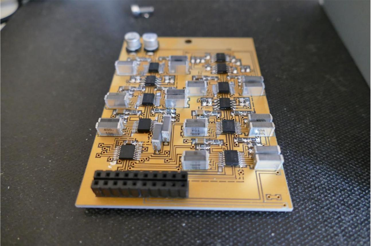
Please notice, that the filterboard connector on filterboards for Tiny LD, is different from other Gotharman instruments. This design choice was made, because there were not enough room in the tiny box, for a standard filterboard connector.
