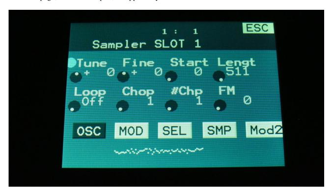
In the bottom of the sampler page, the selected samplings waveform is shown in rough graphics. When the sample, or part of it, is played back, the indicator below the waveform will show the current playback point.
