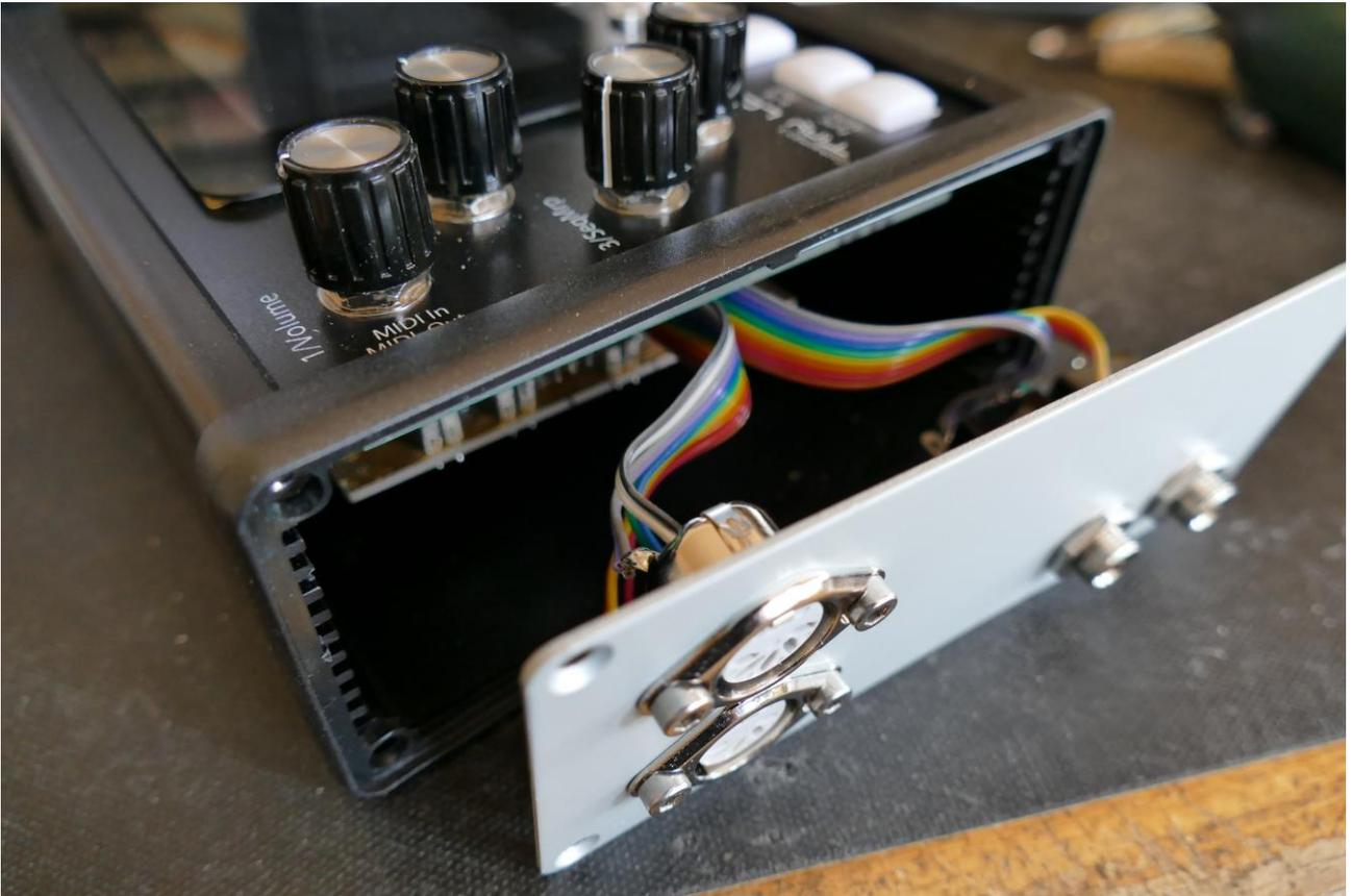
Mount the left end panel, and put the 4 screws back:
