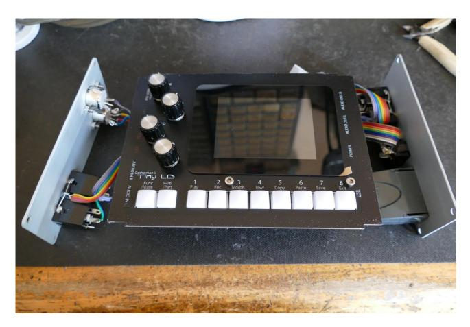
Slide the front panel into the box, from the right, towards left. Again, hold the left end panel, so that it stays inside the box, to prevent scratching the top of the box.
