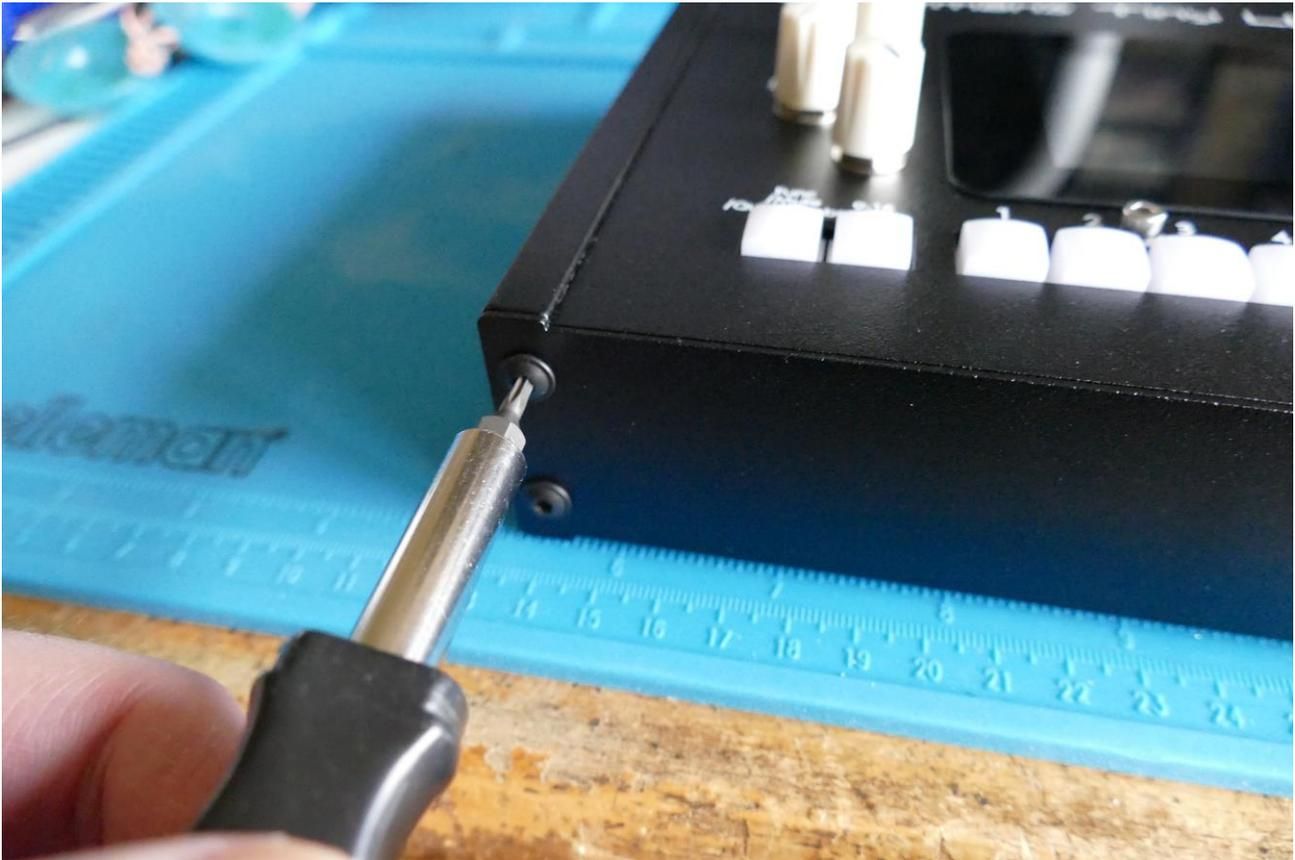
Remove the 2 hex screws located on the left side of the front facing panel, using a T10 Torx.
