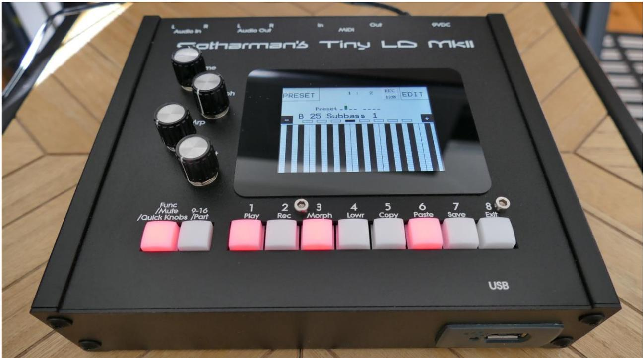
On the front facing panel, you will find the USB connector. This supports USB MIDI, USB CV and a USB FLASH drive can be connected.
