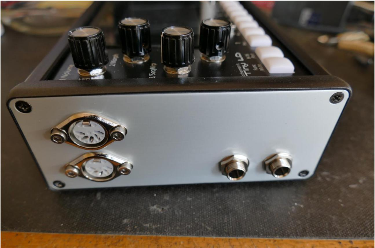
On the left end panel of your Tiny LD, you will find the stereo audio inputs and MIDI in and out.
