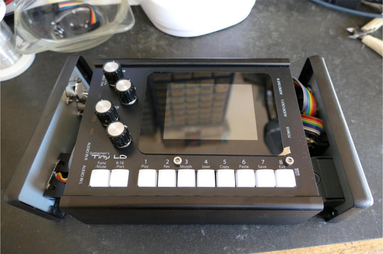
Remove the plastic frames from the end panels.
