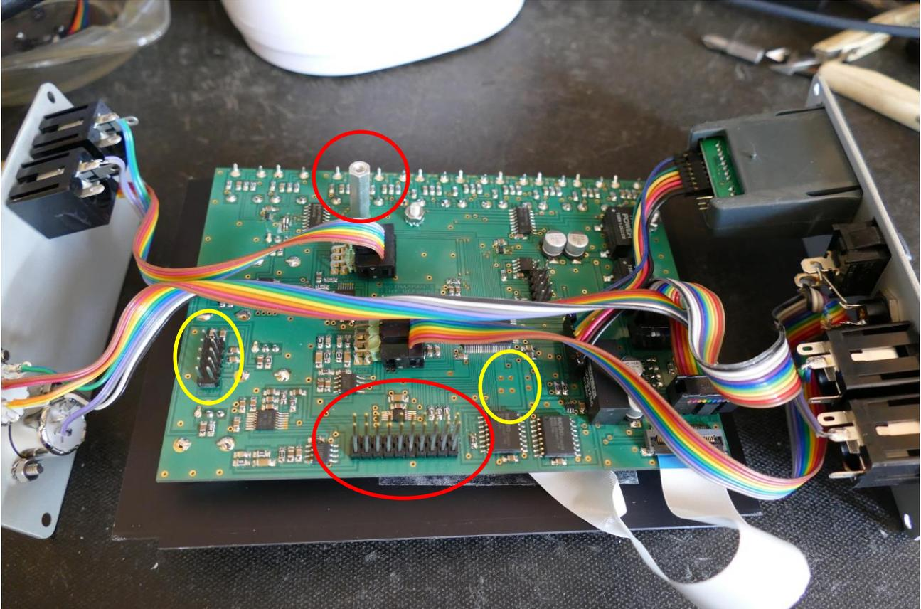
The connector and the spacer in the red circles, is where you will need to place the filterboard.
