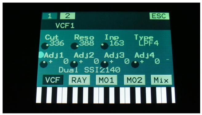
Each edit page has up to 8 parameters, that can be edited. The parameters are shown on the display as 8 parameter names, each with an alphanumeric value below them, that shows the current value of the parameter.
