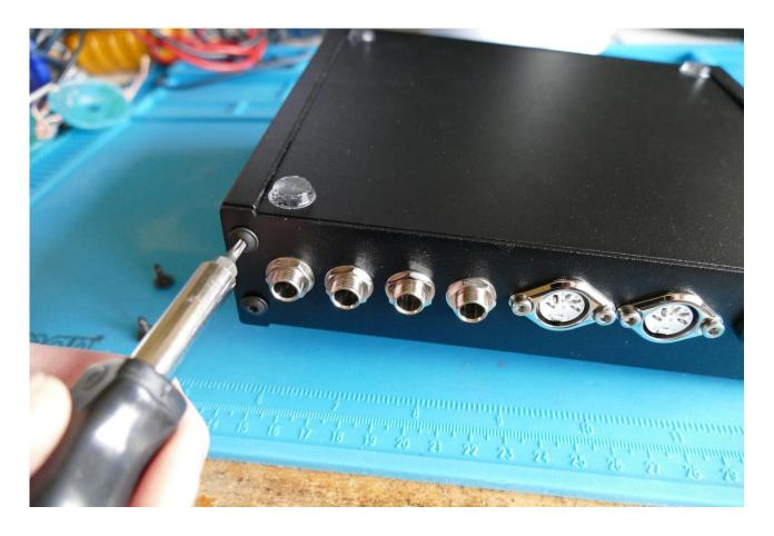
Mount the hex screws. You will need to hold the end panel in place, when you are mounting these screws.
