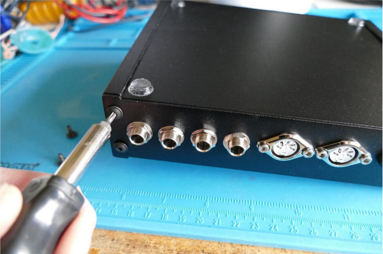
Mount the hex screws. You will need to hold the end panel in place, when you are mounting these screws.
