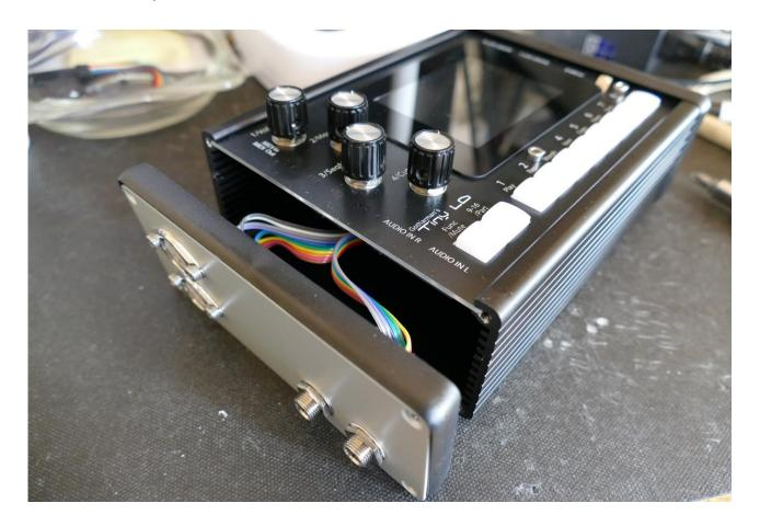
Turn your Tiny LD around, and remove the 4 screws in the corners of the right end panel, again using the Phillips screwdriver.
