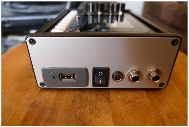
On the right end panel of your Tiny LD, you will find the power switch, connection for power supply, stereo audio outputs, and USB.
