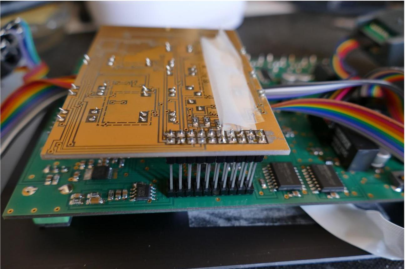
Place a nylon washer between the filterboard and the PCB spacer, that is holding it. Put the screw, with nylon and shakeproof washer mounted on top of the spacer, and tighten it.
