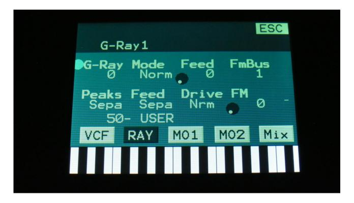
On the second VCF edit page (RAY), you will find the G-Ray and FM parameters as usual, plus you will be able to select how parameter 2 and 4 should interact with parameter 1 (the Peaks and Feed switches in this example). You will also be able to select, if audio output 2 of the filter, should be normal or inverted (the Drive parameter in this example).
