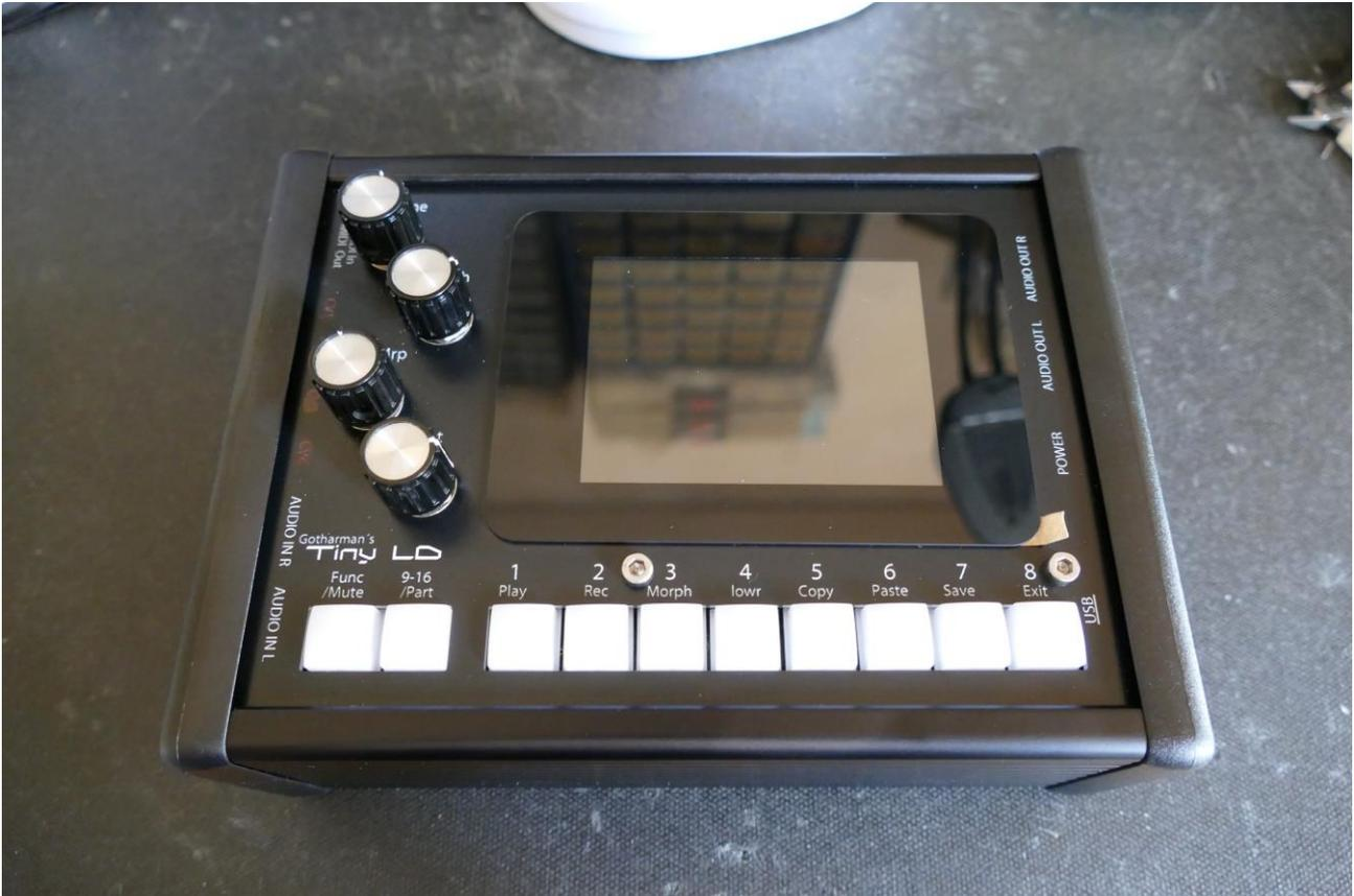
Remove the 4 screws in the corners of the left end panel, using the Phillips screwdriver.
