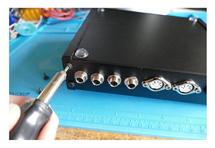
Remove the 2 hex screws, that are now on the left side of the rear panel, using a T10 Torx.
