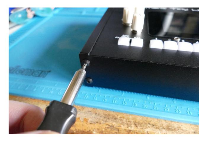
Remove the 2 hex screws located on the left side of the front facing panel, using a T10 Torx.
