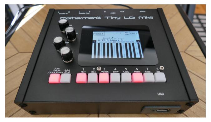
On the front facing panel, you will find the USB connector. This supports USB MIDI, USB CV and a USB FLASH drive can be connected.
