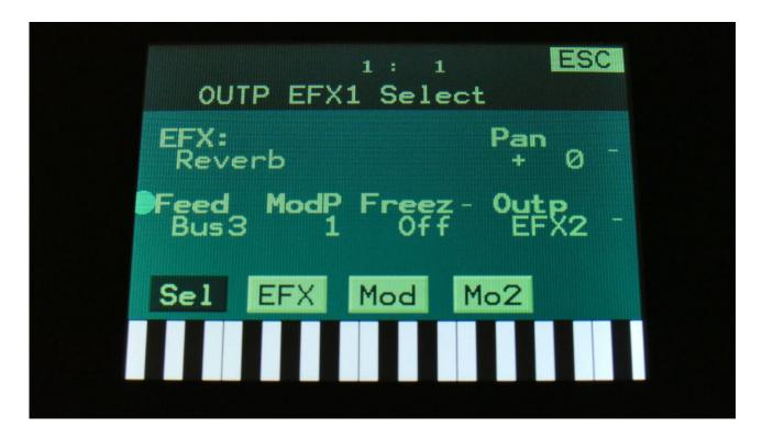
By this parameter, it is possible to send the audio output of Output Effect 1 to either the left and right audio outputs, by setting it to **L+R**, or to Output Effect 2, by setting it to **EFX2**, for serial connection of the 2 Output Effects.
