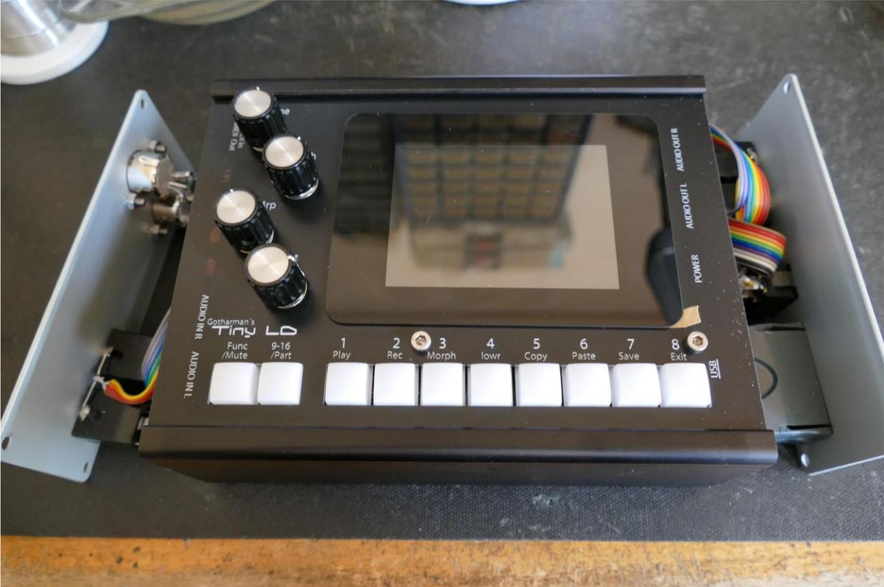
Now carefully slide the front panel towards the right, while navigating the left end panel, to stay inside the box, in order not to scratch the top of the box.
