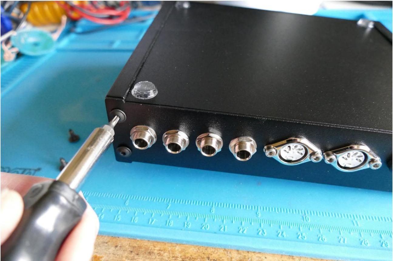
Remove the 2 hex screws, that are now on the left side of the rear panel, using a T10 Torx.
