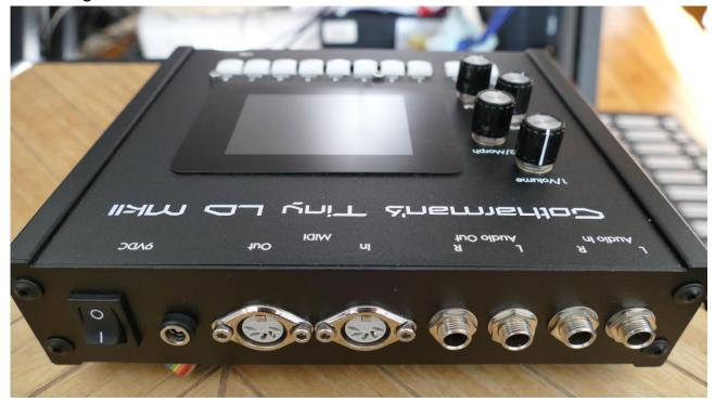
On the rear panel of your Tiny LD MkII, you will find the power switch, connection for power supply, MIDI in and out, and stereo audio inputs and outputs.
