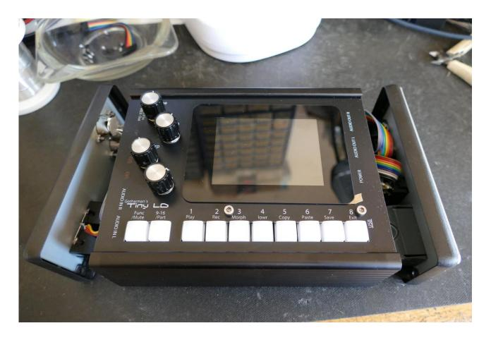
Remove the plastic frames from the end panels.
