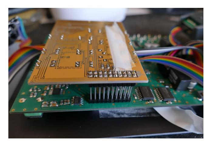
Place a nylon washer between the filterboard and the PCB spacer, that is holding it. Put the screw, with nylon and shakeproof washer mounted on top of the spacer, and tighten it.
