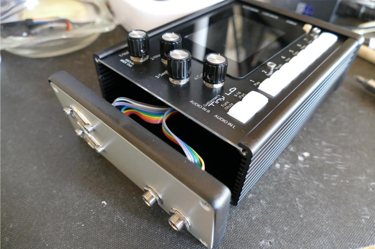
Turn your Tiny LD around, and remove the 4 screws in the corners of the right end panel, again using the Phillips screwdriver.
