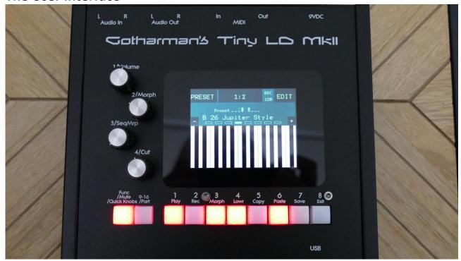
Tiny LD has a highly sensitive and responsive capacitive touch display, 8 step/trigger/part select/function buttons, a Func/Mute button, and a Steps/Parts 9-16 select/Part Select button. It has 4 Edit Knobs for controlling and editing parameters and sending MIDI CC's, that doubles as Volume, Morph and sequencer Morph knobs. Only Edit Knob 4/Cut are assignable, to control other parameters.
