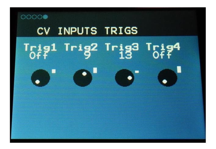
Trig1, Trig2, Trig3, Trig4: Off, 1-16. Sets up the CV inputs to trigger specific parts.
