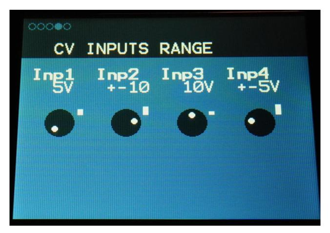
**Inp1, Inp2, Inp3, Inp4:** Sets the input voltage range of the CV inputs. The CV input range should be set for each input, to match the connected source. Possible voltage ranges are:
