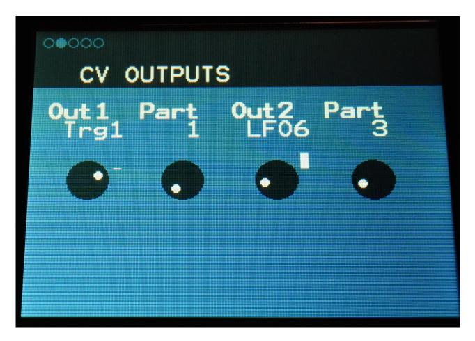
**Out1, Out2:** Selects the modulation source for each CV output. For a complete list of modulation sources, see the list in the user manual.
