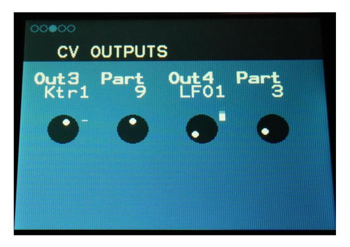
**Out3, Out4:** Selects the modulation source for each CV output. For a complete list of modulation sources, see the list in the user manual.
