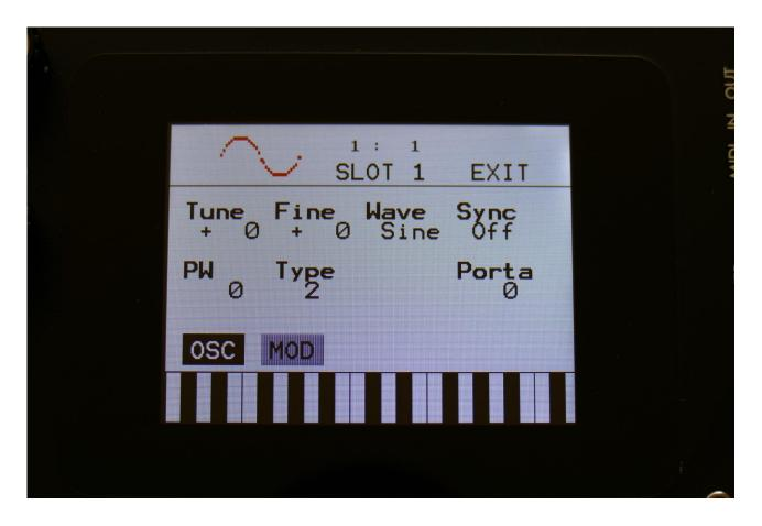
In the middle of the oscillator page, the current waveform is shown.
