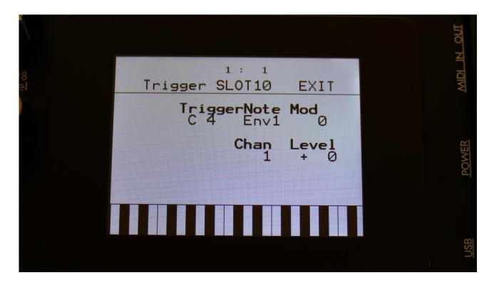
**TriggerNote:** C-1 to G9. The note that will be sent via MIDI out, when the step buttons are in trigger mode (when both the Func/Mute button and the Steps/Part button are unlit), and you push the trigger button, for this part.
