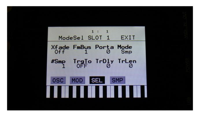
Set Osc1 in sampler mode, and touch the SMP touch button to select the sampling, that you just wave chopped (or any other sampling that you have wave chopped).
