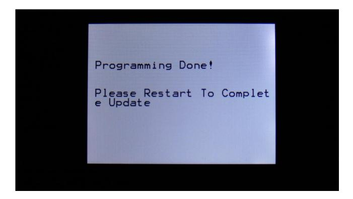
16. When you turn on LD3 after an update, it will need to finalize this. It will show this by turning 10 step button LED's on and off sequentially, one by one. After it has done this for a little while, it will start normally and are ready to use.
