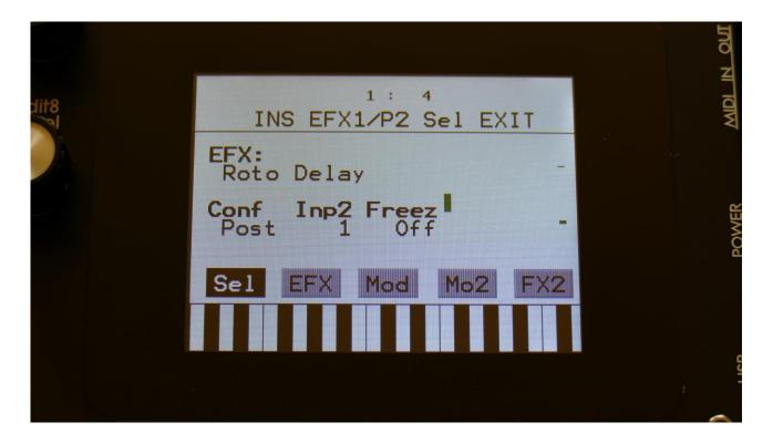
Touch the SEL touch button, to enter the effect select page. Touch FX2/FX1 to jump between insert effect 1 and 2.
