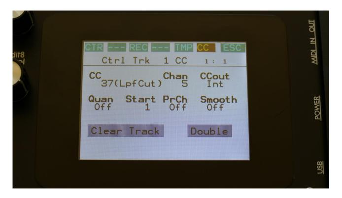
The CC parameter can be set to any MIDI CC between 1 and 122. In the top position, you will find CV In 1 to 4 and Pitch Bend, and at position 16 (CC16), you will find the touch screen keyboard Y-position.
