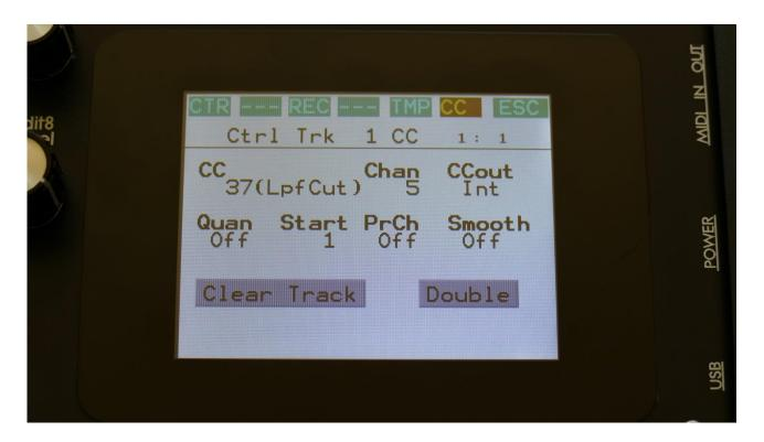
Set the CC parameter, to the parameter, that you want to control with the controller track. A shorted version of the parameter name, will be written in parenthesis.
