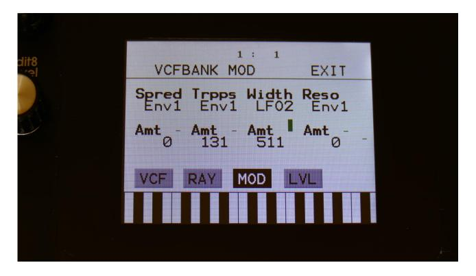
**Spred:** Will modulate the cutoff frequency spread of the filters.
