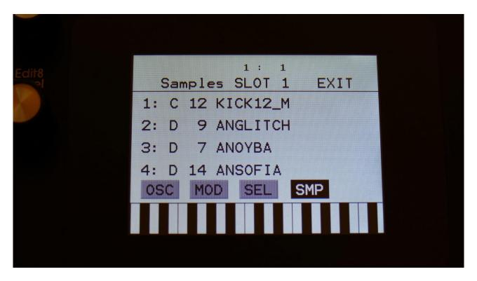
Here you can select 4 samplings for the part. The number of these samplings, that are used, is set by the #Smp parameter on the SEL page. The 4 samples can be selected to play back, setting the Chop parameter, and by chop select modulation.
