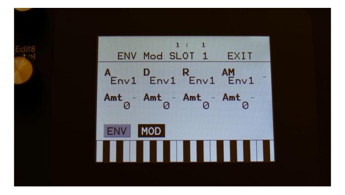
Touch the MOD touch button, to enter the envelope modulation page. OR: Push and release the Func/Mute button, so that it lights up, and push step button 9/Env 2 times.
