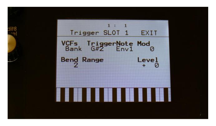
A new parameter, **VCFs**, has been added to this page. Set this to **Part**, to place the analog filters as part filters, for part 1 to 6. Set it to **Bank**, to put Spazeboard6 in FilterBank mode. To edit the parameters of the filterbank, simply enter the HPF/LPF pages, where the parameters for the analog filters were placed in VCF part mode.
