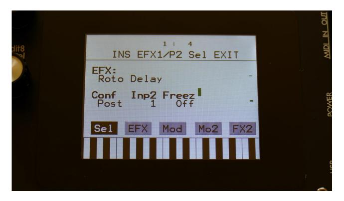
To switch between Insert effect 1 and 2 of the part, touch the FX2/FX1 touch button in the lower right corner of the screen.
