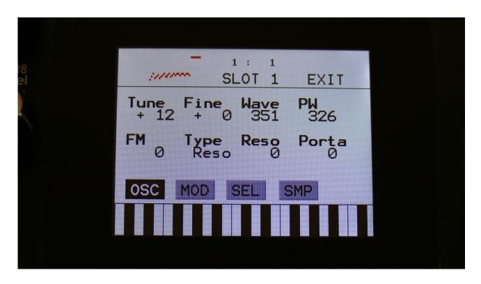
The oscillator1 are the first block in the audio chain of a part. This is, together with Oscillator2, responsible for generating the basic sound of each part, that can be modulated, filtered and effected, for shaping a sound.
