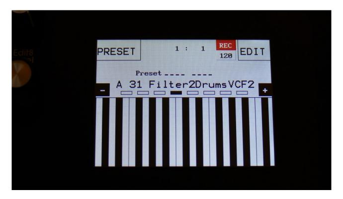
LD3 will now show the Preset select page. The REC indicator on the preset select page, has now turned red, indicating that LD3 is in recording mode. Song realtime recording can also be switched on or off, by touching the REC indicator.
