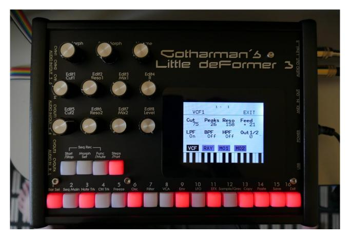
LD3 has a highly sensitive and responsive capacitive touch display, 16 step/trigger/part select/quick jump buttons, a Morph Set button, a Func/Mute button, a Steps/Part button and a Sequencer Start/Stop button. It has 8 Edit/Quick Edit Knobs for controlling and editing parameters and sending MIDI CC's, a (synth) Morph knob, a Sequencer Morph knob and a volume knob.
