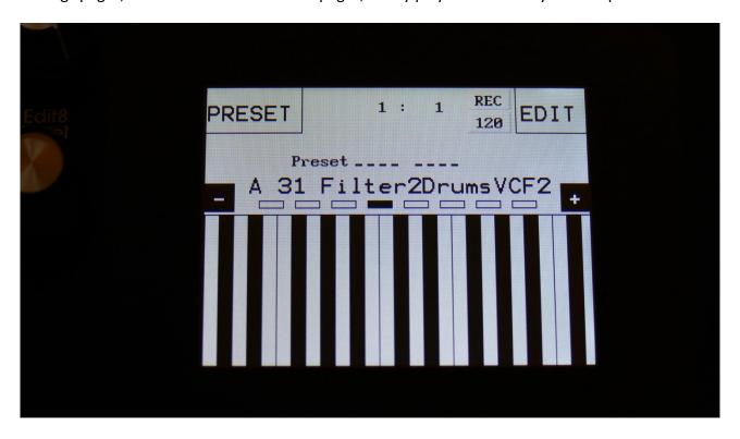
On the Preset and Song Select pages, it is, besides from playing notes on the touch keyboard, also possible to apply modulation to the sound, by placing your finger on different positions between the top and the bottom of the keyboard. This is referred to as Keyboard Y modulation. On any other pages, the keyboard only plays notes.
