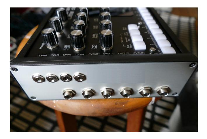
On the left end panel of your LD3, you will find the stereo audio inputs. The optional extra separate audio outputs and the CV inputs are also found here, if installed.
