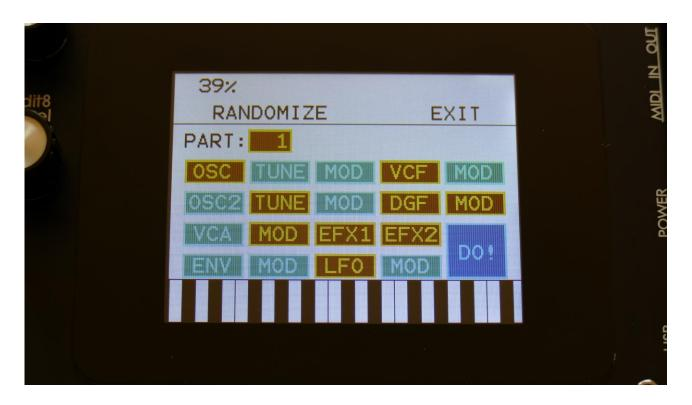
Select the part that you would like to randomize, in the same way as you would usually select a part, by pushing and holding the Steps/Part button, while pressing one of the first 8 step buttons. Switch the blocks on, that you would like to randomize, simply by touching these, adjust the percentage, that it must maximum change the parameters, using Edit Knob 1, and hit "DO!".
