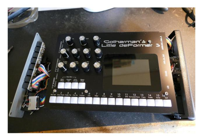
Slide the front panel into the box, from the right, towards left. Again, hold the left end panel, so that it stays inside the box, to prevent scratching the top of the box.
