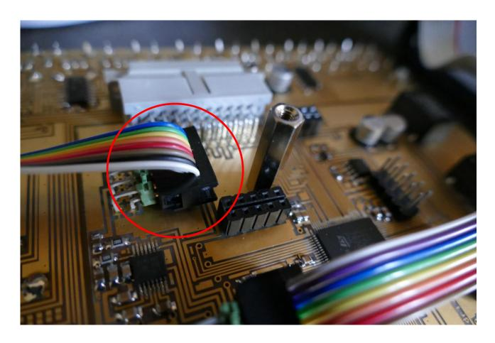
If a screw is located on the spacer on the main board, remove this, so that the spacer looks like on the picture.
