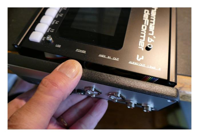
Remove the plastic frame from the left end panel.
