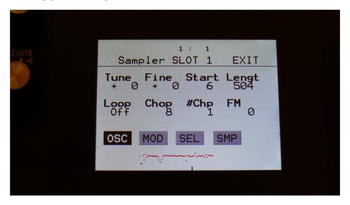
In the bottom of the sampler page, the selected samplings waveform is shown in rough graphics. When the sample, or part of it, is played back, the small black line below the waveform will show the current playback point.
