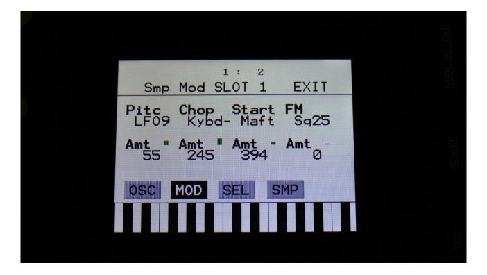
Unlike most other parameters in LD3, only positive modulation are applied to the Chop parameter. So the Chop parameter selects the lowest possible chop to be played back.
