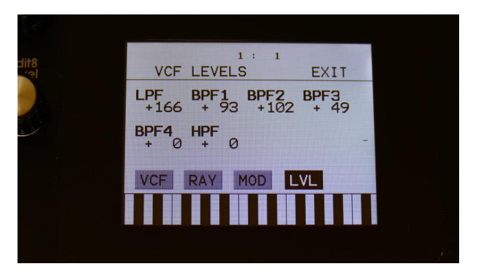
Here you can attenuate (negative value) or boost (positive value) the output levels of each filter separately.
