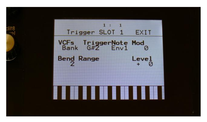
**VCFs:** The analog filters can be arranged as either part filters (Part) or as one big filterbank (Bank). This is described in the analog filters section, later in this manual.
