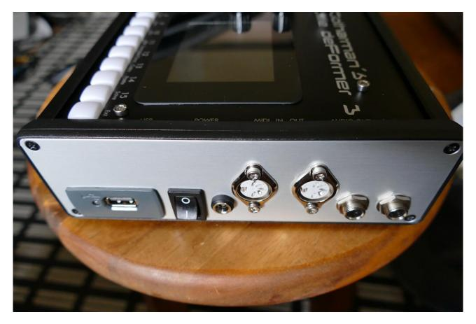
On the right end panel of your LD3, you will find the power switch, connection for power supply, stereo audio outputs, USB, and MIDI in and out.
