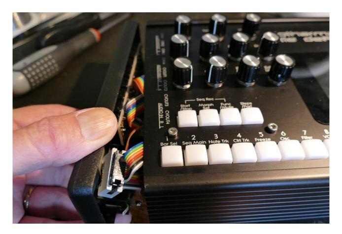
Turn your LD3 around, and remove the 4 screws in the corners of the right end panel, again using the Phillips screwdriver.
