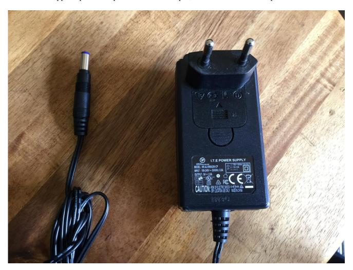
It's a 9V, minimum 2.0A type with a 2.1 mm DC plug, with positive middle. The powersupply on the picture is only for reference. The actual one might look different.
