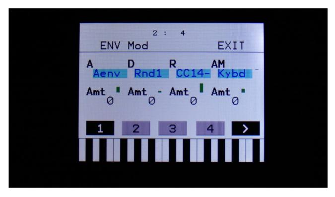
The VU-meter at the right of the screen, shows the Envelope output. The small VU-meters next to the parameters, shows the activity of the selected modulation sources.
