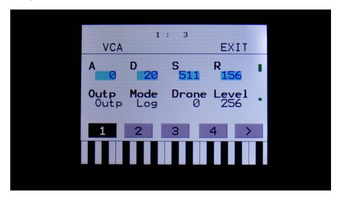
By touching the buttons numbered 1 to 4, the VCA's of part 1 to 4 is selected. In some play modes, it is not possible to edit all parts separately, and only the parts that can be selected, will be shown. Touch the arrow button, to enter other VCA pages, like Modulation.
