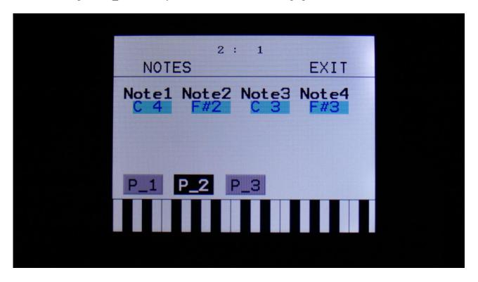
**Note1**, **Note2**, **Note3**, **Note4**: Sets the note number that each trigger button should send each of the 4 parts, when pushed. This setting only affects when the trigger buttons theselves are pushed, not when a trigger is controlled via MIDI, touch keyboard or sequencer.
