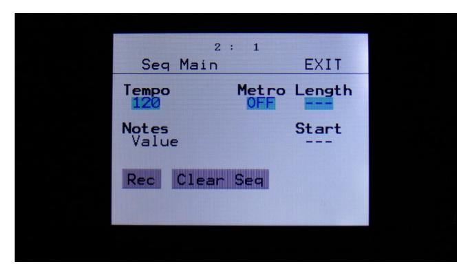
If the tracks lengths and start steps has been set up individually on each track, the global Length and Start steps will no longer be shown as a value, but just as 3 lines.
