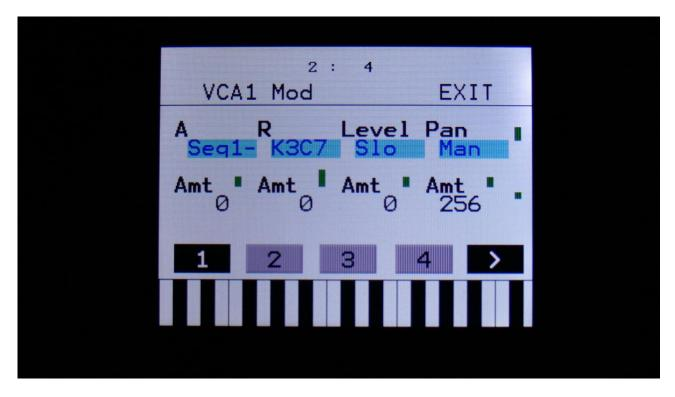
The 2 VU-meters at the right of the screen, shows the VCA input and output. The small VU-meters next to the parameters, shows the activity of the selected modulation sources.
