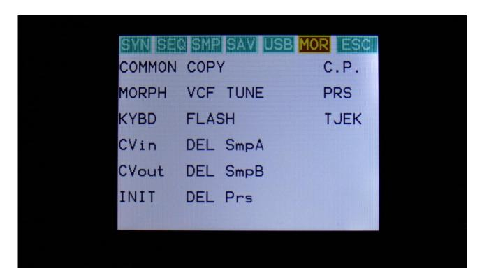
This will get you to the More... page. Here you can set up all the basic PolySpaze B things, like MIDI channel, morphing, touch keyboard and CV in's/out's, make the analog filter tune, check and erase the PolySpaze B memory, initialize the preset and change to song mode.
