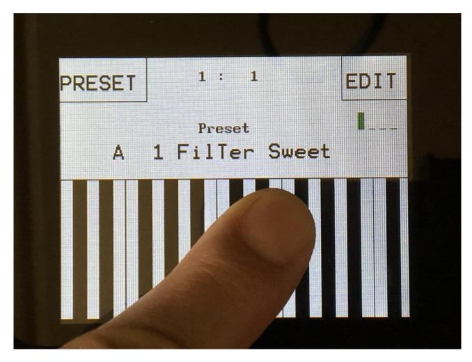
On the Preset and Song Select pages, it is, besides from playing notes on the touch keyboard, also possible to apply modulation to the sound, by placing your finger on different positions between the top and the bottom of the keyboard. This is referred to as Keyboard Y modulation. On any other pages, the keyboard only plays notes.
