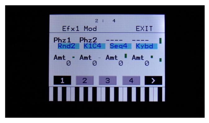
The 2 VU-meters at the right of the screen, shows the Effect input and output. The small VU-meters next to the parameters, shows the activity of the selected modulation sources.
