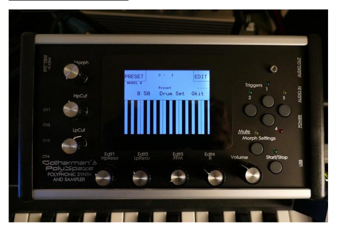
To start and stop sequencer play back, you must push the "Start/Stop" button. When the green LED above the Start/Stop button lights up, it is indicating, that the sequencer is playing back. When the green LED above the Start/Stop button does not light up, the sequencer playback is stopped.
