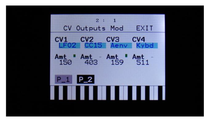
Here you can, with the upper row of parameters selected, by Edit Knob 1 to 4, select the modulation source for each CV output. For a complete list of modulation sources, see the list in the start of the synth section in this manual.
