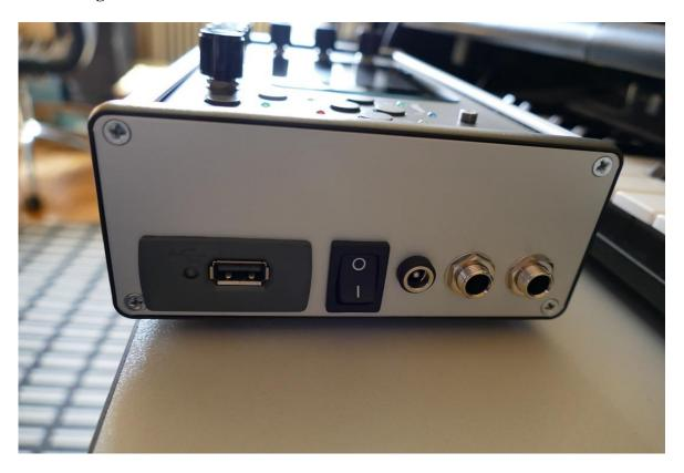
On the right end panel of your PolySpaze B, you will find the power switch, connection for power supply, stereo audio input and output, and USB. The audio inputs and outputs are stereo jacks.
