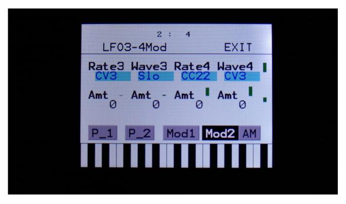
The 2 VU-meter at the right of the screen, shows the LFO outputs. The small VU-meters next to the parameters, shows the activity of the selected modulation sources.
