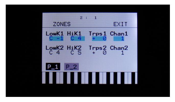
In this block you can set up the key zones and MIDI channels for each of the 4 Synth parts. These zones are effective only when PolySpaze B are in Multi-Timbral and MultiBank play modes, and are controlled from an external MIDI device or from the touch screen keyboard. It is also possible to transpose the incoming notes individually for each zone. Zones can overlap each other.
