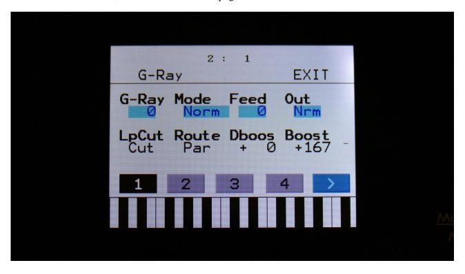
**G-Ray:** Adjusts the amount of g-RAY intermodulation. 0: no g-RAY, 3: max g-RAY. Range: 0 to 3.
