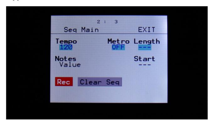
The Rec button turns red, when the Sequencer are in realtime record mode.
