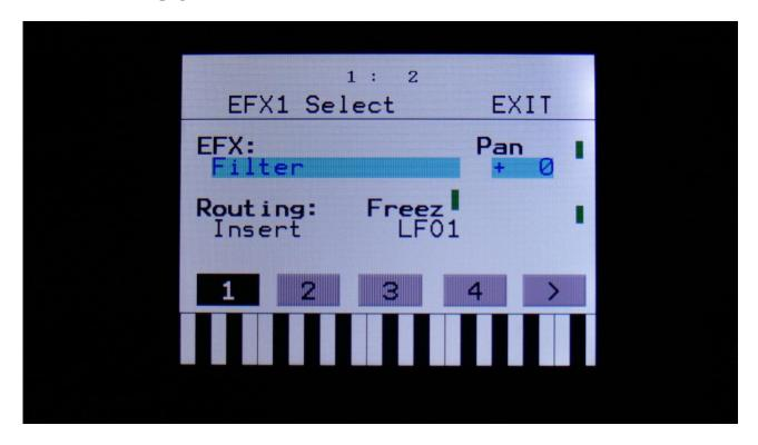
By touching the buttons numbered 1 to 4, the Effects's of part 1 to 4 is selected. In some play modes, it is not possible to edit all parts separately, and only the parts that can be selected, will be shown.
