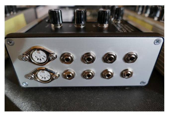
On the left end panel of your PolySpaze B, you will find the MIDI in and out connectors. The optional CV inputs and outputs are also found here, if installed. Please notice, that the upper row of CV connectors are the outputs, and the lower row are the inputs. The upper MIDI connector are the input, and the lower are the output.
