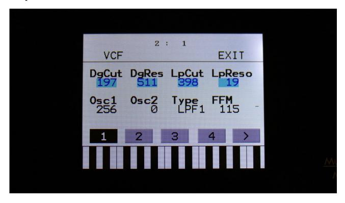
By touching the buttons numbered 1 to 4, the filters of part 1 to 4 is selected. In some play modes, it is not possible to edit all parts separately, and only the parts that can be selected, will be shown. Touch the arrow button, to enter other filter pages, like Modulation and G-Ray.
