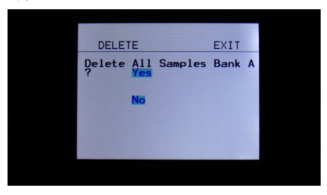
If you are really sure, that you absolutely have to do this, touch "Yes" to start the erase. The sample bank will now be completely wiped out. While it is being erased, PolySpaze B's 5 button LED's will run a sequence. When the LED's shuts off, the erase has been done, and PolySpaze B will return to the More... screen.
