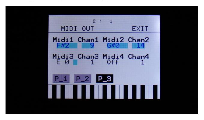
On this page it is possible to select a MIDI note number and a MIDI channel, that will be transmitted via MIDI out, when a trigger button is pushed. When a trigger button is set up to transmit a MIDI note, the sequencer track attached to that trigger, will also transmit MIDI notes on the same MIDI channel.
