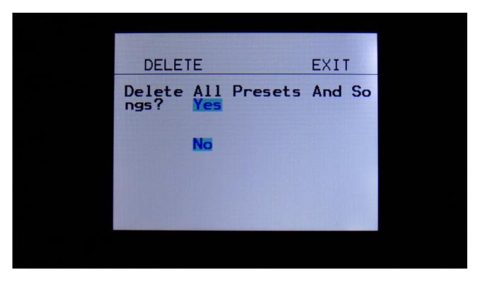
If you are really sure, that you absolutely have to do this, touch "Yes" to start the erase. All presets and songs will now be completely wiped out. While these are being erased, PolySpaze B's 5 button LED's will run a sequence. When the LED's shuts off, the erase has been done, and PolySpaze B will return to the More... screen.
