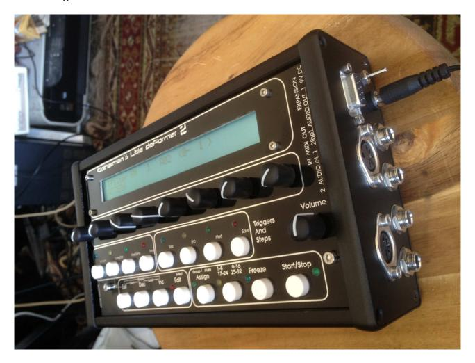
On the right end panel of your Little deFormer, you will find the power switch and connections for power supply, audio inputs and outputs, MIDI in and out and for an expansion box.
