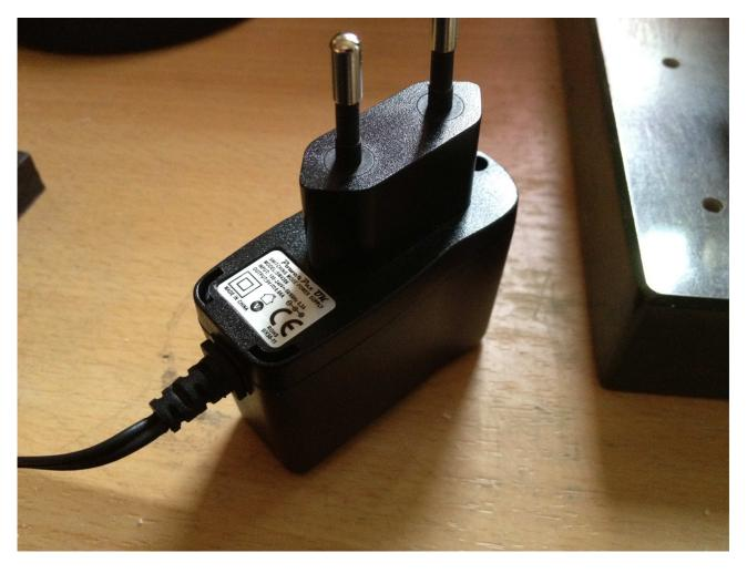
It's a 9V, 660 mA type with a 2.1 mm DC plug, with positive middle.
