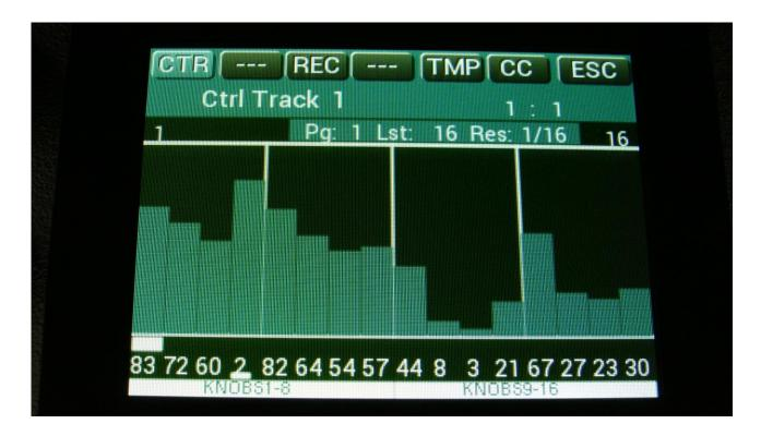
To enter the draw mode, on the controller track values page, touch the CTR field in the upper left corner.
