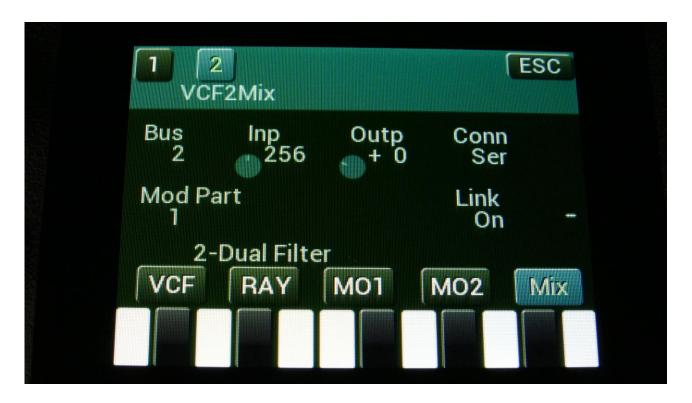
Now all analog filter 2 parameters, except for the Bus parameter, are controlled by analog filter 1.
