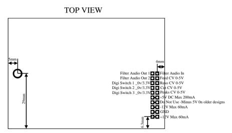
FilterBoard connector: 10 pos, 2 row angled connector with 2.54mm pitch like the SSW-110-02-G-D-RA.
