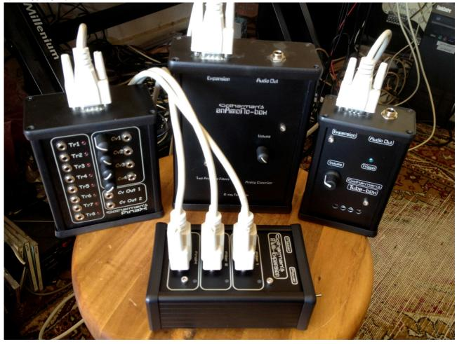
The audio signal sent to the filter expansion boxes, are sent before Little deFormers effects. If you would like to add effects to the filter treated signals, or if you would like to use this setup, with only one pair of outputs, you can connect the audio outputs of the 2 filter boxes to Little deFormers 2 inputs. Please remember that you must turn the input levels of both the inputs up, in Little
