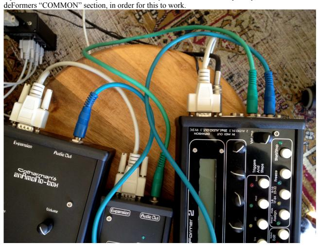
Now connect the expansion cable, supplied with Multi-Expansion, from Little deFormer's Expansion connector to Multi-Expansion's "Master" connector.
