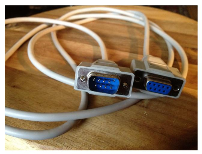
If you should need a longer cable, or if your cable one day gets lost, you can use a 1:1, 9-pin SUB-D cable. If you have a Little deFormer 1, just notice, that like on the picture, pin 5 of the male connector must be cutted. This is because, on some Little deFormers, pin 5 on the expansion connector are connected to its audio path, and if this pin on the cable are connected, it will create a lot of noise on the audio. If you have a Little deFormer 2, you can just use the SUB-D cable as it is.
