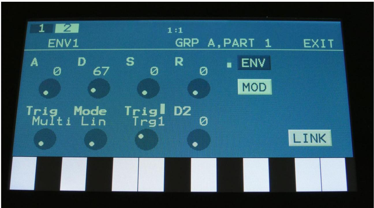
Each group has 2 envelope modules (8 in total), each with an ADSR envelope and a Decay envelope. The ADSR envelope can run in various linear and logarithmic modes, the envelope time can be timed by 4, for long envelope times, and the ADS segment can be looped. The envelopes can be triggered by any sources. The A, D, R and output amount parameters can be modulated. Envelope 2, the decay envelope, is always linear. When the ADSR Envelope is looped, the Decay envelope is looped in sync with this.
