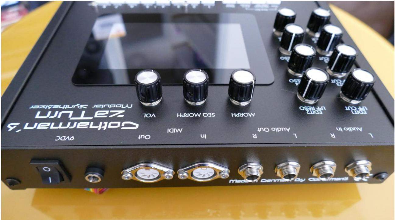
On the back panel of your Zatur, you will find the power switch, connection for power supply, audio inputs and outputs and MIDI in and out.
