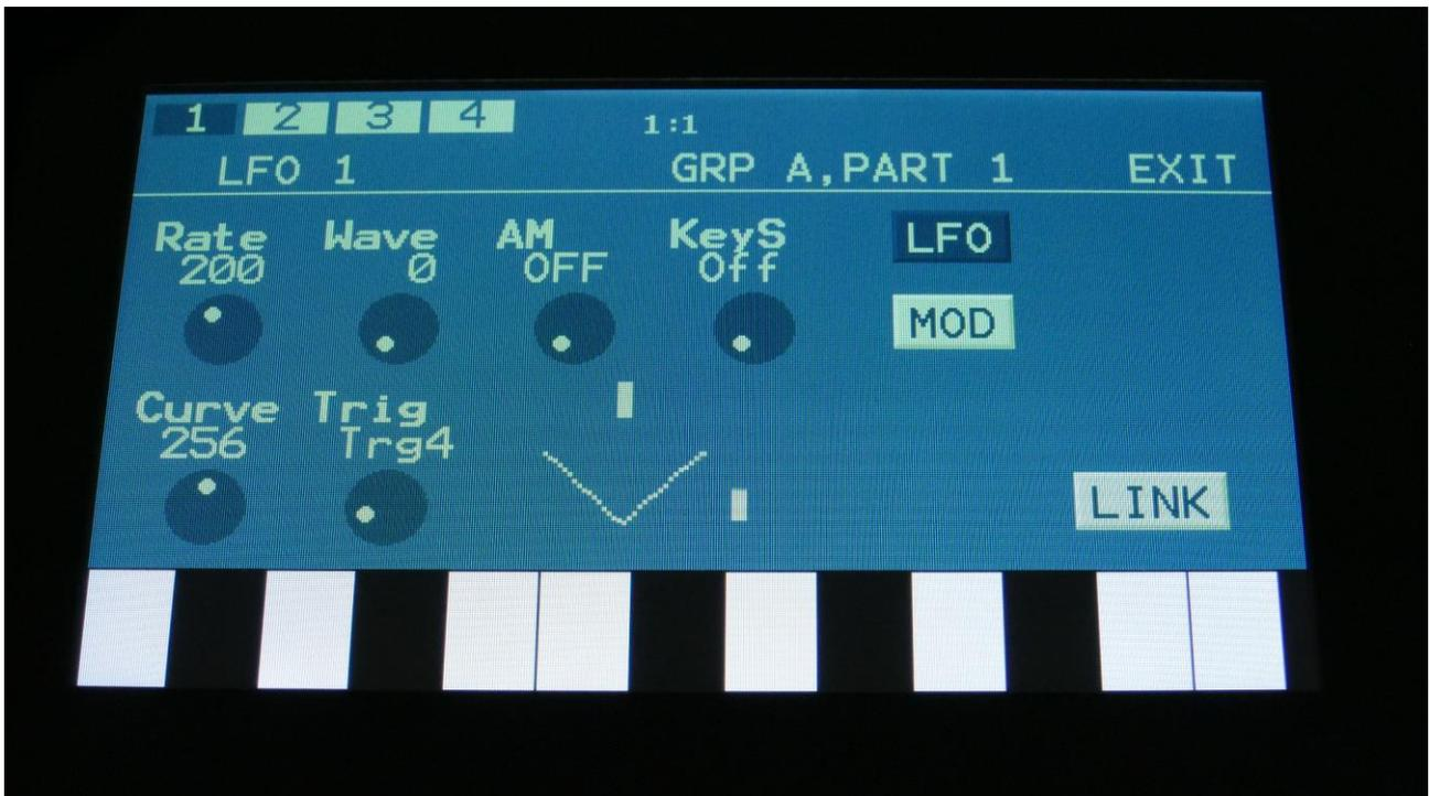
Each group has 4 LFO's (16 in total) with a waveform that morphs from triangle to sawtooth to pulse to FM waves. Curve can be adjusted from logarithmic to linear to exponential. The LFO's can be key synced, and a one-shot mode is available, for using the LFO's as envelopes. The Rate, Wave and Curve parameters can be modulated.
