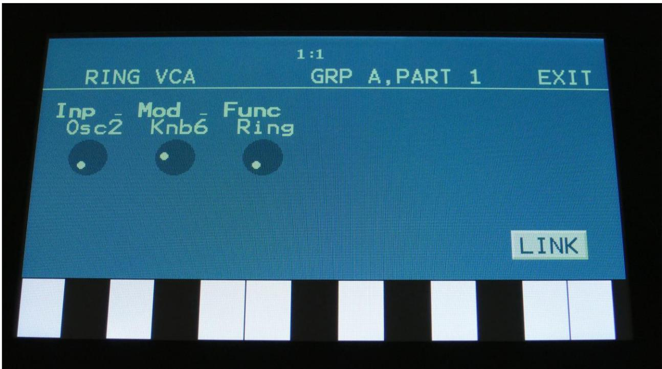
Each group has one Ring VCA (4 in total), which can be used as both VCA's, Ring Modulators, as logic modules and as mixers.
