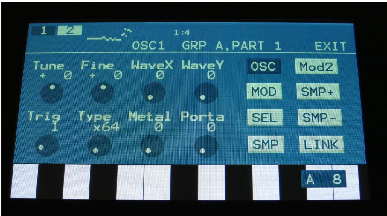
Each group has 2 of these oscillators (8 in total), which can run in several different modes, for maximum flexibility. The outputs of the oscillators can be connected to any audio and modulation inputs. To select a specific oscillator, first select the group/part, and then touch the numbers in the upper right corner.
