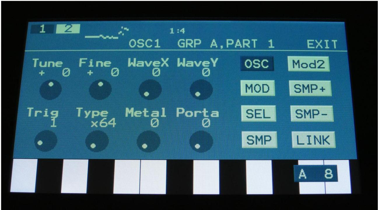
In the upper left corner of the oscillator page, the currently generated waveform is shown.
