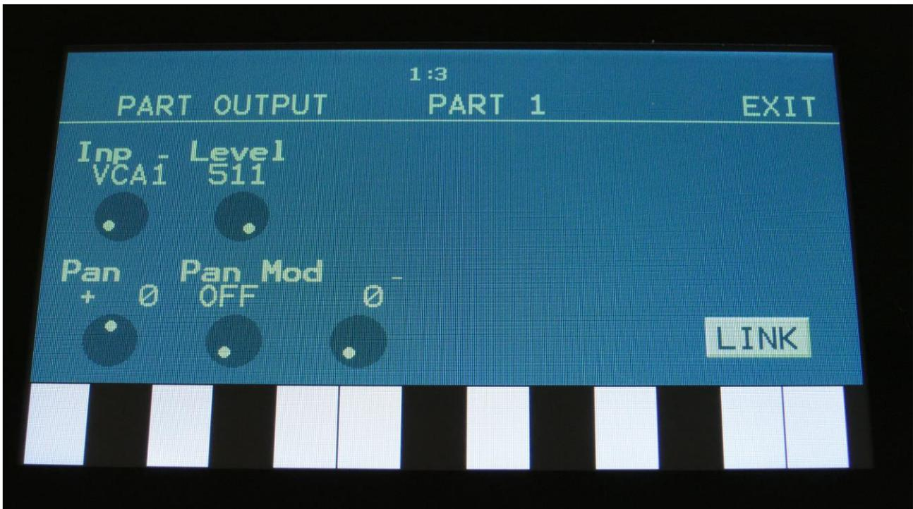
In the output module, signals from any modules can be assigned and routed to the audio outputs. Panning of sounds and pan modulation is also done here.
