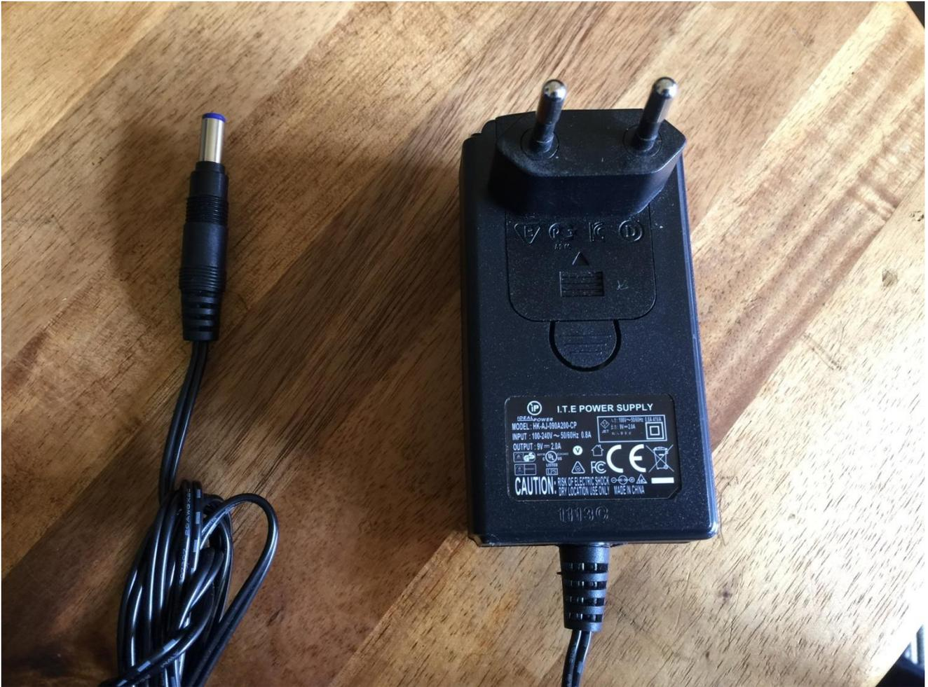
It's a 9V, minimum 2.0A type with a 2.1 mm DC plug, with positive middle. The power supply on the picture is only for reference. The actual one might look different.
