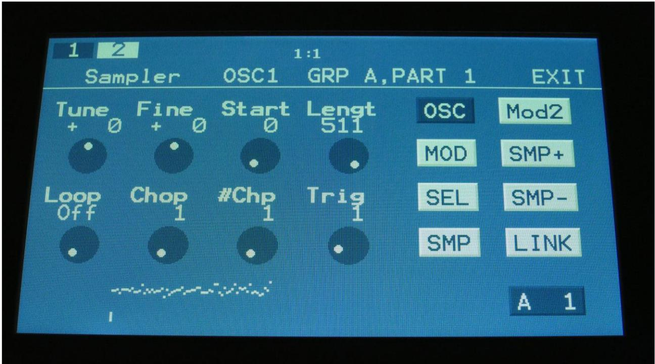
In the bottom of the sampler page, the selected samplings waveform is shown in rough graphics. When the sample, or part of it, is played back, the small black line below the waveform will show the current playback point.
