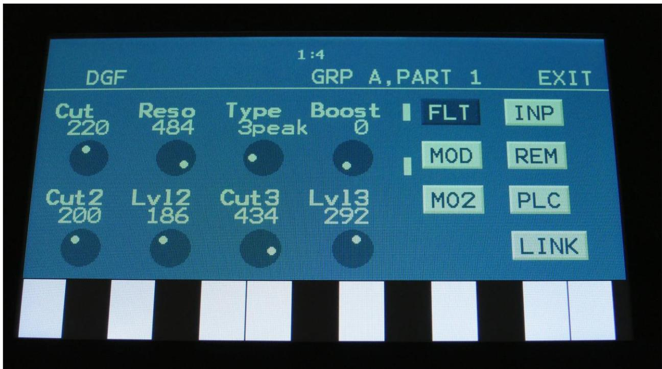
The 8 digital filters on Zaturm have 27 different filter types to choose from. Cutoff frequencies, resonance and triple filter levels can be adjusted and modulated.
