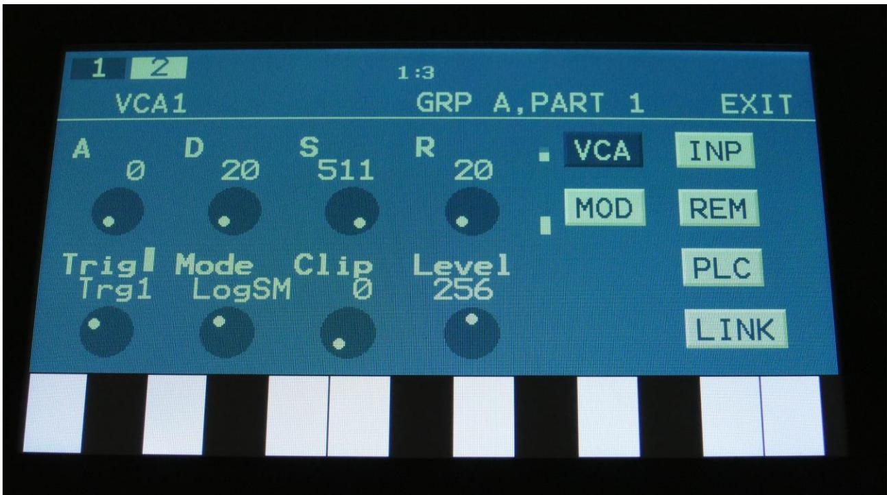
Each group of Zaturm has 2 VCA's (8 in total) with built-in ADSR Envelopes and an envelope Clip parameter, that adds more punch to the VCA. The VCA's has 16 different linear and logarithmic modes (characteristics), and the envelope time can be timed by 4, for long envelope times. The VCA envelopes can be triggered by any sources. The A, D, R and output level parameters can be modulated.
