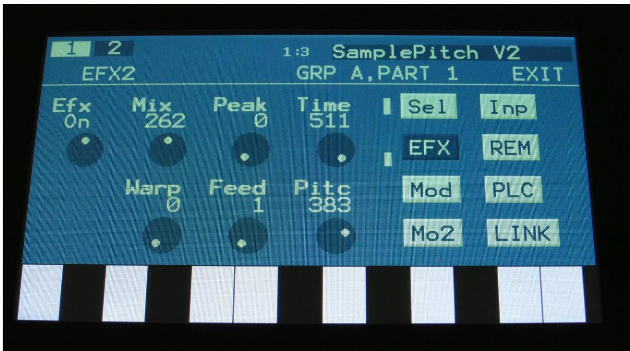
Zaturm has 8 effect processors, 2 in each group, EFX 1 and 2. All effect types are available in both EFX 1 and 2, but EFX 2 has some additional “large” effects, like reverb and granulators. Most parameters can be modulated. Zaturm has many of the classic deFormer effect, but also some new ones, like a wavefolder and some new pitch effects.
