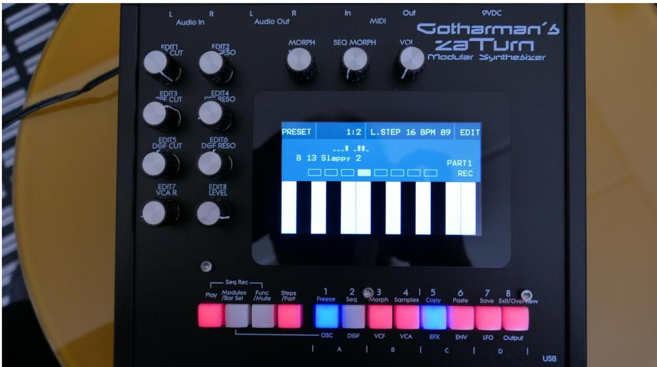
Zaturn has a highly sensitive and responsive capacitive touch display, 8 step/trigger/part select/quick jump buttons, a Modules/Bar Sel button, a Func/Mute button, a Steps/Part button and a Sequencer Play button. It has 8 Edit/Quick Edit Knobs for controlling and editing parameters and sending MIDI CC's, a (synth) Morph knob, a Sequencer Morph knob and a volume knob.
