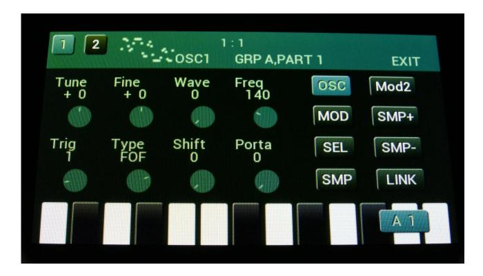
Wave: Morphs the basic tone between sine wave and triangle wave.
