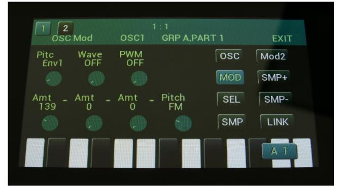
When an Oscillator pitch modulation mode is set to PM, the Pitc2 parameters name is changed to Phase.
