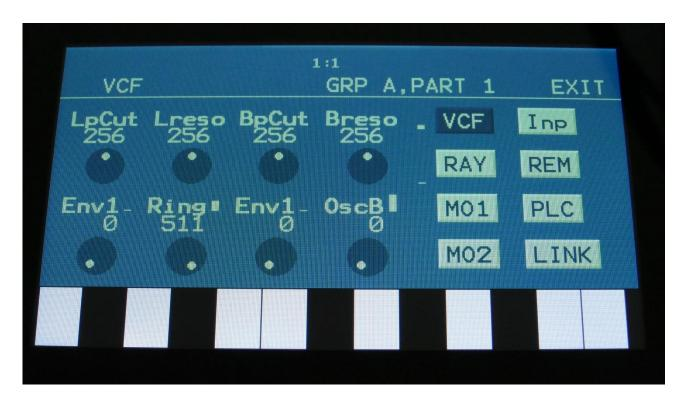
The parameters are exactly the same as for the original zaTurn filters, except for that the BPF can be switched to a HPF, and that the LPF slope can be set.
