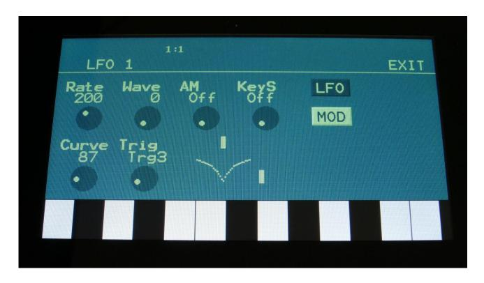
A trigger output parameter has been added to each LFO.
