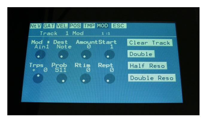
2 new functions have been added to the sequencer note tracks MOD page: Half Reso (half resolution) and Double Reso (double resolution).
