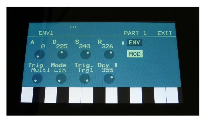
An output VU-meter has now been added to the Decay Envelope, near the Dcy parameter.
