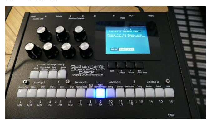
Now the selected bank will be shown on the step buttons, by one step button lighting up. Push a step button to select another bank.
