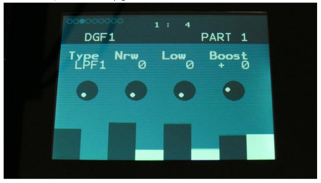
**Type:** Sets the DGF1 filter type. See the list of filter types.
