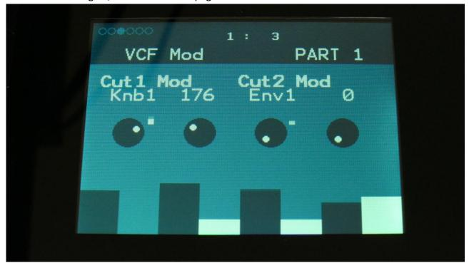
**Cut 1 Mod:** Select a modulation source and adjust the amount of modulation for the Cut parameters. This can affect the cutoff frequency of both analog filters, one of them, or they can be modulated inverted to each other. This can be set, using the Mod1 parameter, explained on one of the next pages. The small VU-meter next to the modulation source selector, shows the output of the selected modulation source.
