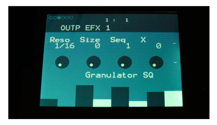
**Reso:** Adjusts the resolution of the sequencer track, that controls the granulator. The granulator only uses the controller values of the sequencer steps, so the controller track and the granulator can run in different resolutions.
