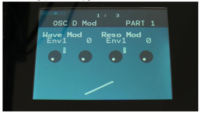
**Wave Mod:** Select a modulation source and adjust the amount of modulation for the Wave parameter. The small VU-meter next to the modulation source selector, shows the output of the selected modulation source.
