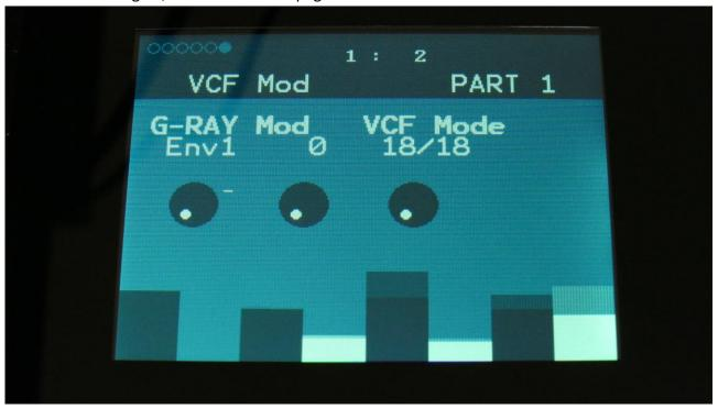
**G-RAY Mod:** Select a modulation source and adjust the amount of modulation for the G-Ray Feed parameter. The small VU-meter next to the modulation source selector, shows the output of the selected modulation source.
