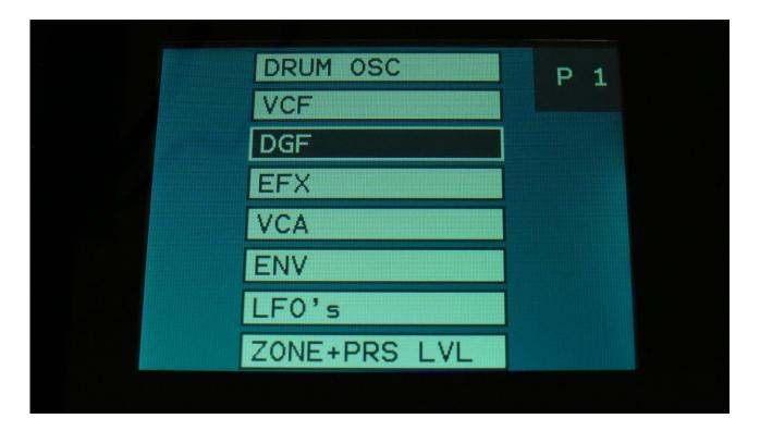
To enter the digital filters, select DGF from the synth modules overview page, using the < and > buttons, and hit the Edit button.
