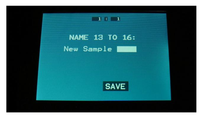
Input the last 4 characters of the name for the new sampling, using Edit Knob 1 to 4.
