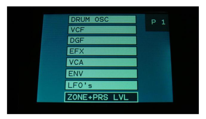
To enter the Zone and Preset Level, select ZONE+PRS LVL from the synth modules overview page, using the < and > buttons, and hit the Edit button, or touch the ZONE+PRS LVL module on SpazeDrum Black.
