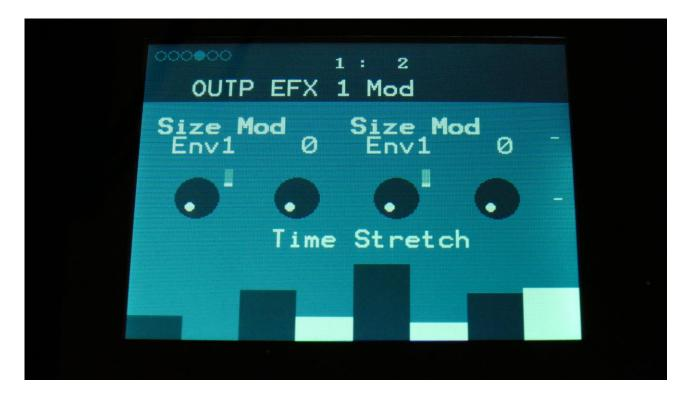
**Size Mod:** Select a modulation source and adjust the amount of modulation for the Size parameter. The small VU-meter next to the modulation source selector, shows the output of the selected modulation source.
