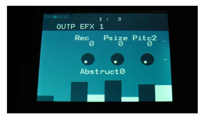
**Rec:** 0 to 511. Sets the record buffer size. Determines for how long time it should record the input, before it starts over again.
