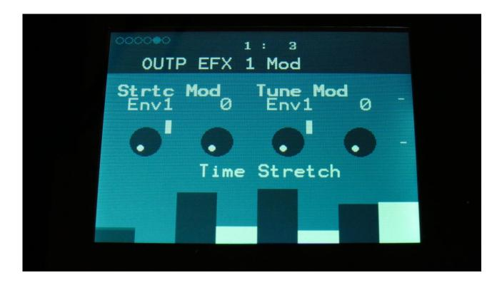
**Strtc Mod:** Select a modulation source and adjust the amount of modulation for the Strtch parameter. The small VU-meter next to the modulation source selector, shows the output of the selected modulation source.
