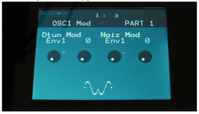
**Dtun Mod:** Select a modulation source and adjust the amount of modulation for the Dtun parameter. The small VU-meter next to the modulation source selector, shows the output of the selected modulation source.
