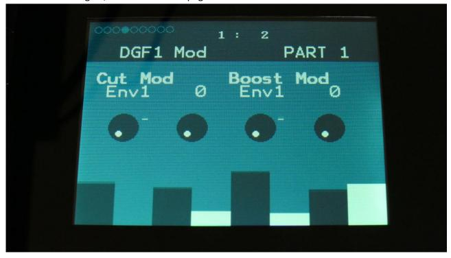
**Cut Mod:** Select a modulation source and adjust the amount of modulation for the DGF1 Cut parameter. The small VU-meter next to the modulation source selector, shows the output of the selected modulation source.
