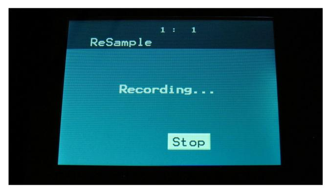
When recording has started, you can leave the ReSample pages, by pushing the Exit button, and go tweak some parameters, while it is recording, if desired.
