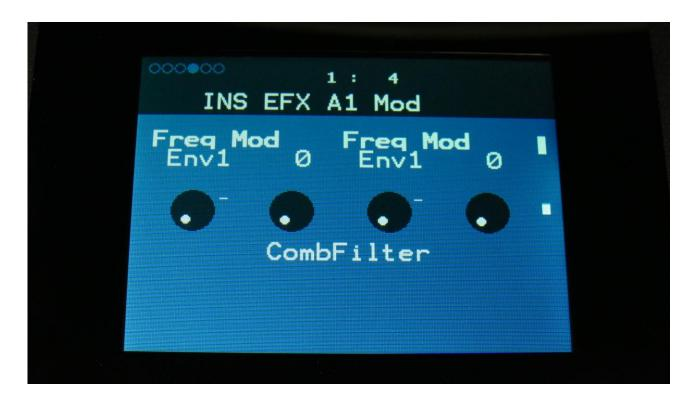
**Freq Mod:** Select a modulation source and adjust the amount of modulation for the Freq parameter. The small VU-meter next to the modulation source selector, shows the output of the selected modulation source.
