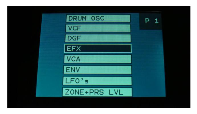
To enter the effects, select EFX from the synth modules overview page, using the < and > buttons, and hit the Edit button, or touch the EFX module on SpazeDrum Black.
