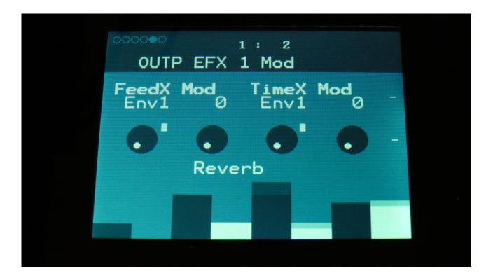
**FeedX Mod:** Select a modulation source and adjust the amount of modulation for the FeedX parameter. The small VU-meter next to the modulation source selector, shows the output of the selected modulation source.
