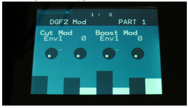
**Cut Mod:** Select a modulation source and adjust the amount of modulation for the DGF2 Cut parameter. The small VU-meter next to the modulation source selector, shows the output of the selected modulation source.
