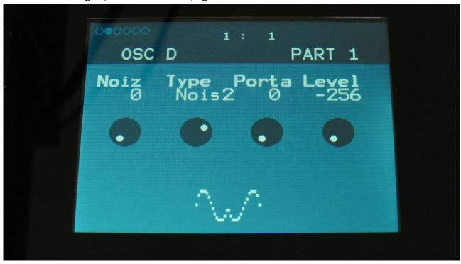
Noiz: Sets the degree of noise feedback, to create different sorts of noise waveforms.
