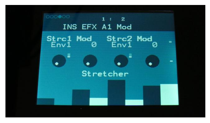
**Strc1 Mod:** Select a modulation source and adjust the amount of modulation for the Strc parameter. The small VU-meter next to the modulation source selector, shows the output of the selected modulation source.
