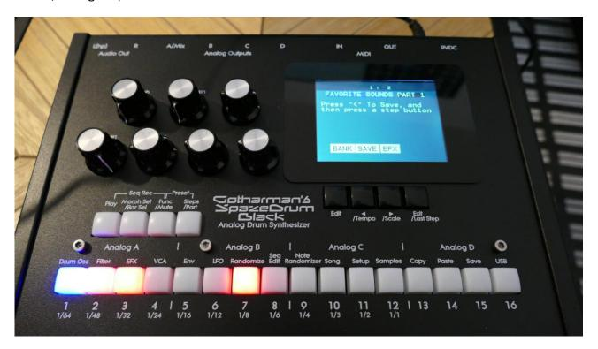
Initially the sounds are loaded without the insert effects settings. To load sounds with the insert effects included, push the > button, or touch the EFX touch button on SpazeDrum Black, so that EFX turns dark blue, and then push a step button, to load a sound. EFX only affects loading of sounds, not saving.
