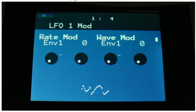
**Rate Mod:** Select a modulation source and adjust the amount of modulation for the Rate parameter. The small VU-meter next to the modulation source selector, shows the output of the selected modulation source.
