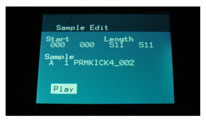
On this page you can audition samples from the FLASH memory, adjust the samples start and end points, and access other sample edit menu's.
