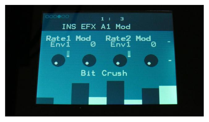
**Rate1 Mod:** Select a modulation source and adjust the amount of modulation for the Rate parameter. The small VU-meter next to the modulation source selector, shows the output of the selected modulation source.
