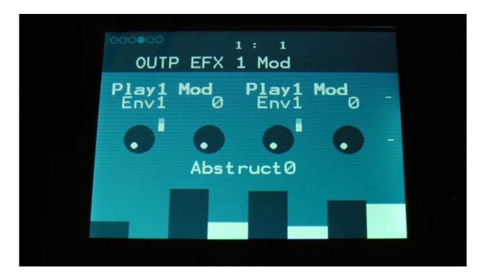
**Play1 Mod:** Select a modulation source and adjust the amount of modulation for the Play1 parameter. The small VU-meter next to the modulation source selector, shows the output of the selected modulation source.
