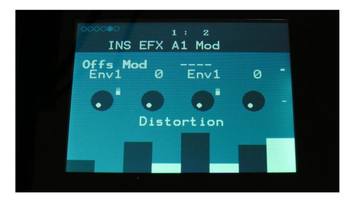
**Offs Mod:** Select a modulation source and adjust the amount of modulation for the Offs parameter. The small VU-meter next to the modulation source selector, shows the output of the selected modulation source.
