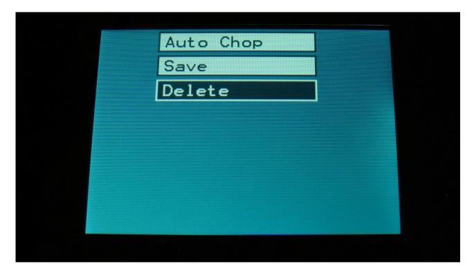
Navigate to Delete, using the < and > buttons, and hit the Edit button, or touch the Delete module on SpazeDrum Black. SpazeDrum will now jump back to the Chop page, and the selected chop point has been deleted.
