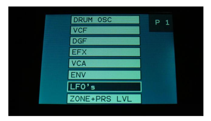
To enter the LFO's, select LFO's from the synth modules overview page, using the < and > buttons, and hit the Edit button, or touch the LFO's module on SpazeDrum Black.
