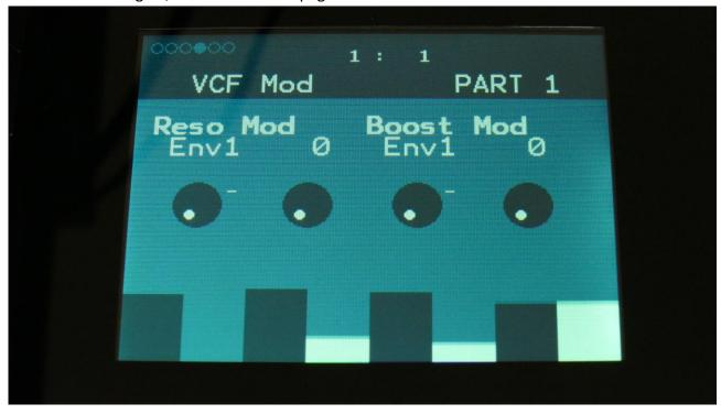
**Reso Mod:** Select a modulation source and adjust the amount of modulation for the Cut parameters. This will affect the resonance of both of the analog filters. The small VU-meter next to the modulation source selector, shows the output of the selected modulation source.
