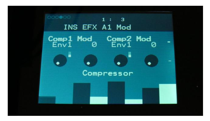
**Comp1 Mod:** Select a modulation source and adjust the amount of modulation for the Comp parameter. The small VU-meter next to the modulation source selector, shows the output of the selected modulation source.
