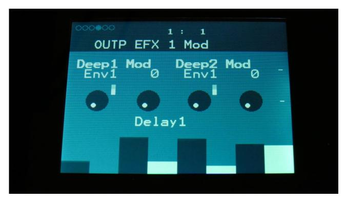
**Deep1 Mod:** Select a modulation source and adjust the amount of modulation for the Deep parameter. The small VU-meter next to the modulation source selector, shows the output of the selected modulation source.
