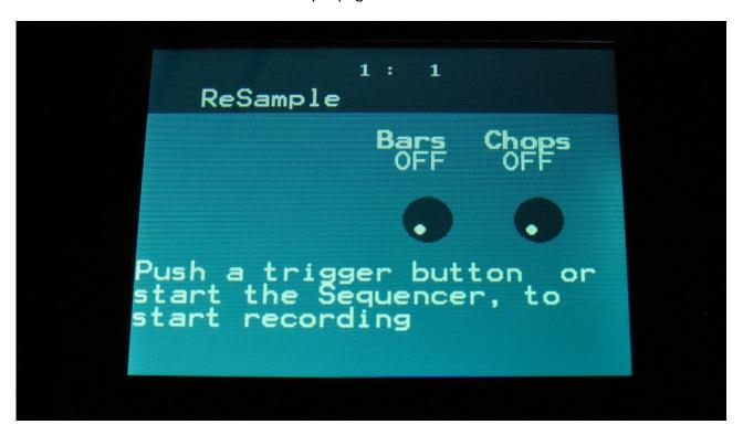
If you would like the sampling to be a specific number of bars, and/or if you would like chops generated while recording, set the desired values, using the Edit Knobs. If you want to manually stop the sampling, and don't need chop points, or will add chop points later, leave both settings to Off.
