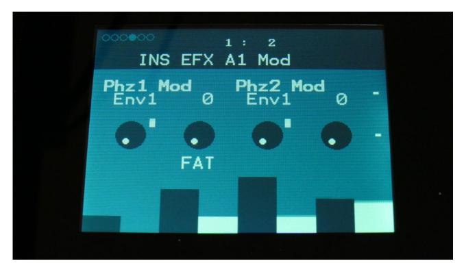
**Phz1 Mod:** Select a modulation source and adjust the amount of modulation for the Phaze parameter. The small VU-meter next to the modulation source selector, shows the output of the selected modulation source.
