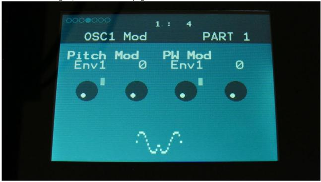
**Pitch Mod:** Select a modulation source and adjust the amount clap envelope speed modulation. The small VU-meter next to the modulation source selector, shows the output of the selected modulation source.
