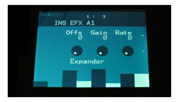
**Offs:** 0 to 511. Sets the level point where the expansion will kick in. The more this is turned up, the higher the input signal will need to be, before it starts to gain.
