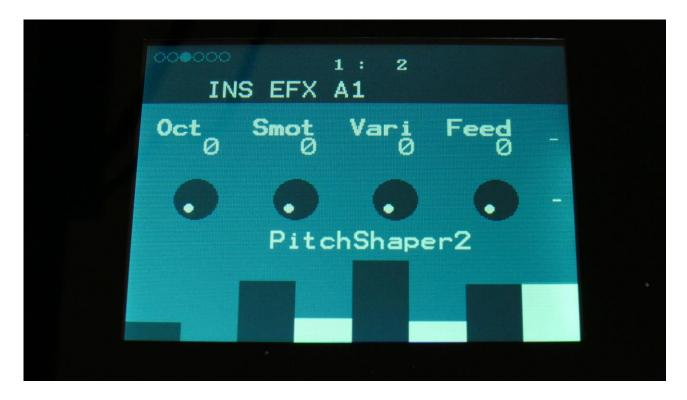
Oct: Octave transpose. From 0 to +3 octaves.
