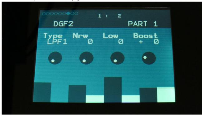
**Type:** Sets the DGF2 filter type. See the list of filter types.
