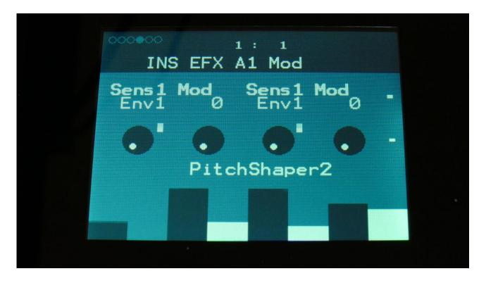
**Sens1 Mod:** Select a modulation source and adjust the amount of modulation for the Sens1 parameter. The small VU-meter next to the modulation source selector, shows the output of the selected modulation source.
