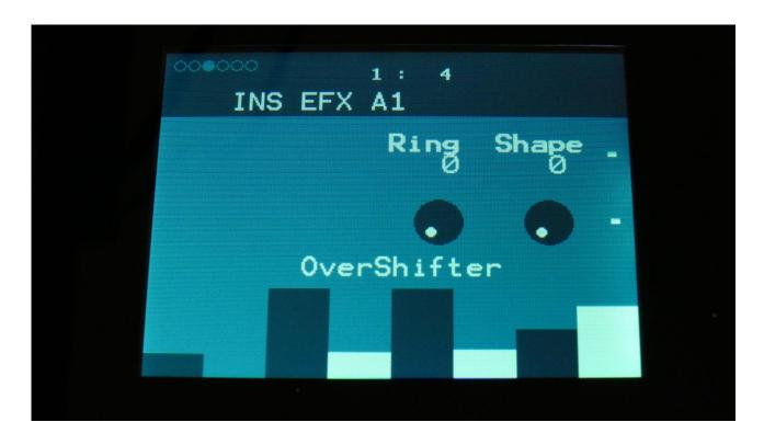
**Ring:** Turning this up will add ringing/metal/noise to the signal.
