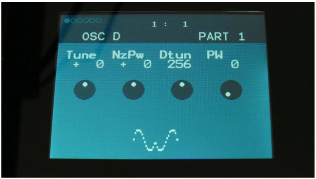
**Tune:** Value -64 to +63. When the Clap oscillator is selected, the Tune parameter sets the speed of the clap envelope.
