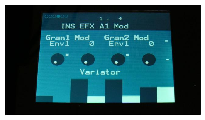
**Gran1 Mod:** Select a modulation source and adjust the amount of modulation for the Gran parameter. The small VU-meter next to the modulation source selector, shows the output of the selected modulation source.
