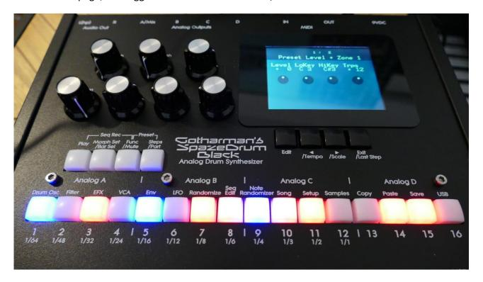
If you don't use, or don't need some of the parts/zones laid out on your MIDI keyboard, you can switch individual zones off, simply by pushing the trigger button, that represents the zone/part, so that it becomes unlit. Switch them back on again, by pushing the trigger button again, so that it lights up. When a zone is switched off, it is completely skipped by the MIDI input, and its assigned notes are used by the zone below it.
