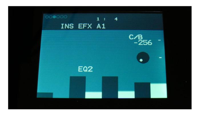
**C/B:** Cut/Boost. Setting this to a negative value, will damp frequencies on the input signal. Setting it to a positive value, will boost frequencies on the input signal.
