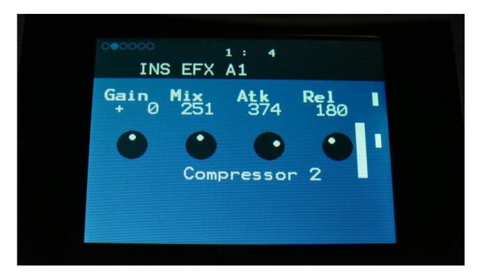
The 2 VU-meters at the right of the screen, shows the Effect input and output. The larger VU-meter illustrates the compressor VCA output level.
