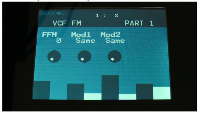
**FFM:** Filter FM. Turning this up will make Oscillator 2 modulate the cutoff frequencies of both of the analog filters.
