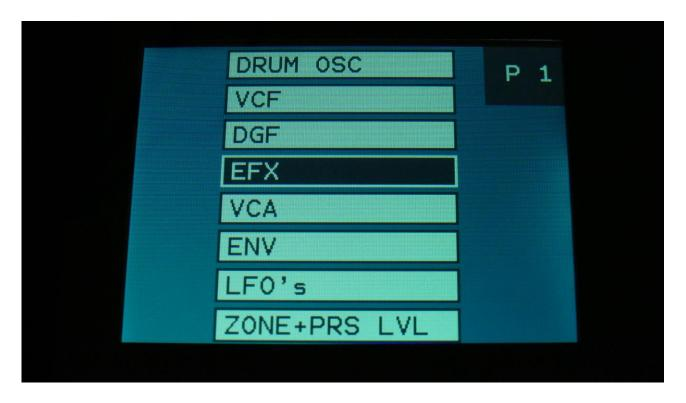
From any drum part, select the EFX module, using the < and > buttons, and push the Edit button, to access the effect pages, or touch the EFX module on SpazeDrum Black.
