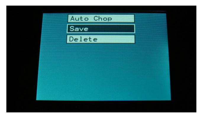
Select Save, using the < and > buttons, and hit the Edit button, or touch the Save module on SpazeDrum Black. Now SpazeDrum will write "Saving Sample..." on the display for a short while, and thereafter return to the Chop page.
