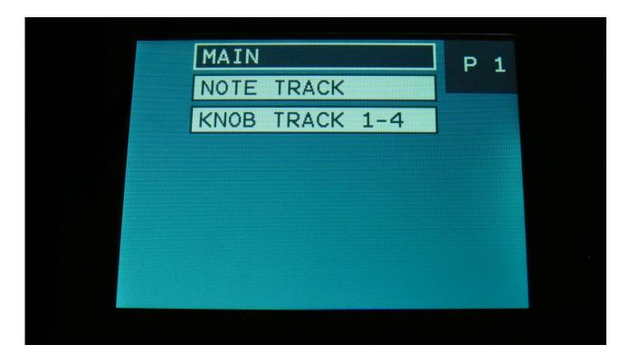
To enter the Sequencer Main page or any of the tracks, simply select the text showing the name of the group that you would like to enter, using the < and > buttons, and then push the Edit button, or touch the MAIN module on SpazeDrum Black.
