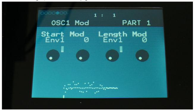
**Start Mod:** Select a modulation source and adjust the amount of modulation for the Start parameter. The small VU-meter next to the modulation source selector, shows the output of the selected modulation source.
