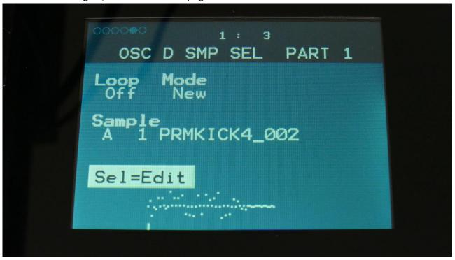
Here you can select the sampling, that oscillator D should play back. To do so, hit the **Edit** button. Now "**Sel=Edit**" will turn dark blue, and you can use the < and > buttons to select the desired sampling. Hold any of these buttons to scroll. When you have selected the desired sampling, simply hit the **Edit** button again. It is also possible to switch sample **loop** on and off, by turning **Edit Knob 1**.
