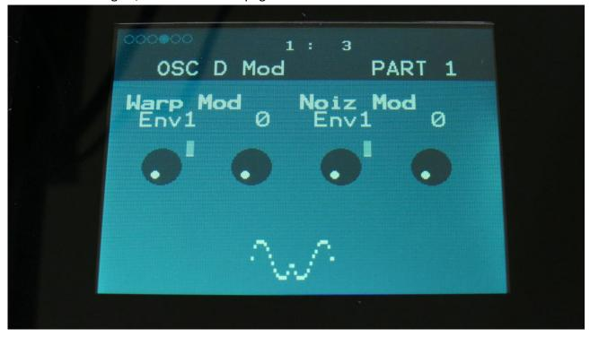
**Warp Mod:** Select a modulation source and adjust the amount of modulation for the Warp parameter. The small VU-meter next to the modulation source selector, shows the output of the selected modulation source.
