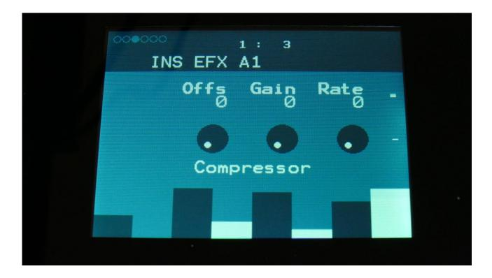
**Offs:** 0 to 511. Sets the level point where the compression will kick in. The more this is turned up, the higher the input signal will need to be, before it starts to compress.
