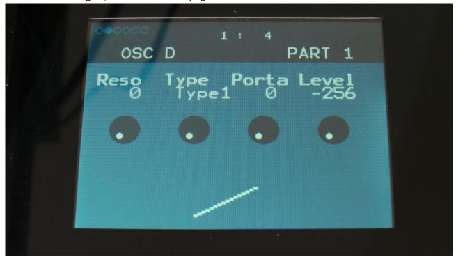
**Reso:** The amount of resonances fed back, when the resonator oscillator type is selected. The higher this parameter is set, the more resonances are fed back into the oscillator. Even at setting zero, some resonances are fed back. Range: 0 to 511.
