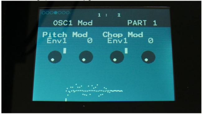
**Pitch Mod:** Select a modulation source and adjust the amount of Oscillator 1 pitch modulation. The small VU-meter next to the modulation source selector, shows the output of the selected modulation source.
