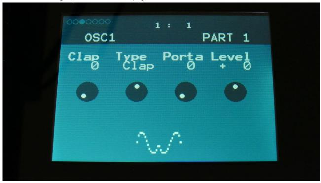
Clap: Value 0 to 511. Sets how much the clap envelope should shape the noise signal.
