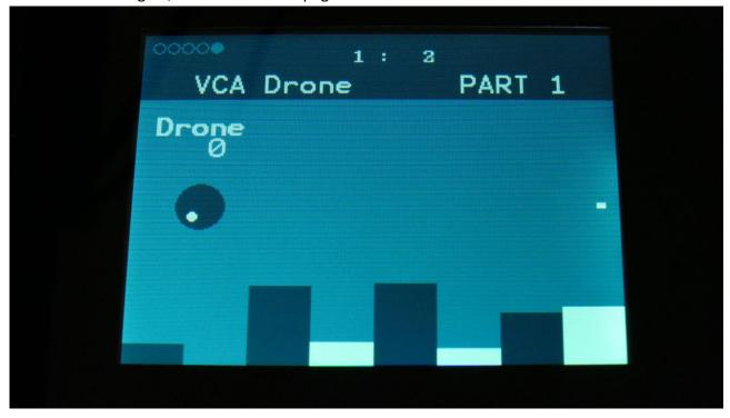
**Drone:** 0 to 511. VCA envelope drone offset level. When this is turned up, the VCA envelope will never reach an output value, lower than what this is adjusted to –It will release to this adjusted value, instead of zero. Use this to keep the output of a synth part open for drone sounds.
