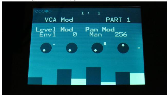
**Level Mod:** Select a modulation source and adjust the amount of modulation for the Level parameter. The small VU-meter next to the modulation source selector, shows the output of the selected modulation source.
