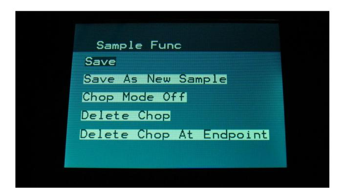
Navigate to "Save As New Sample", using the < and > buttons, and push the Edit button.
