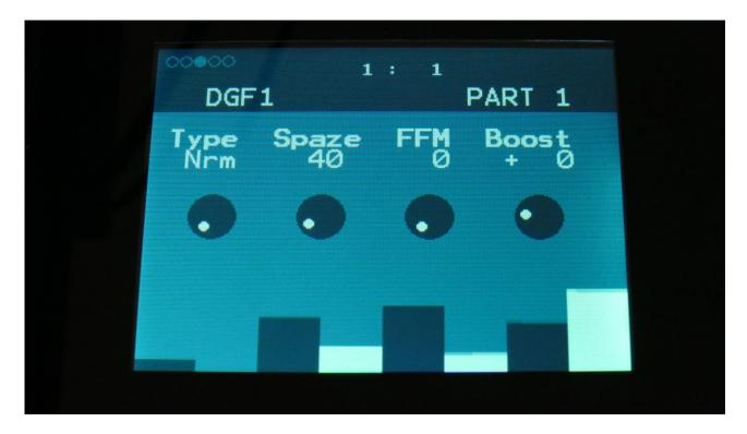
**Type:** Sets the filter type. **Nrm:** Standard triple filters. **Sharp:** Sharp triple filters with narrow frequency bands.
