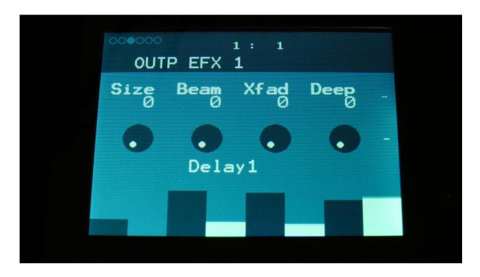
**Size:** A granular parameter. The more this is turned up, the less space of the delay box is used, causing some echo's to repeat, and others not to sound at all.
