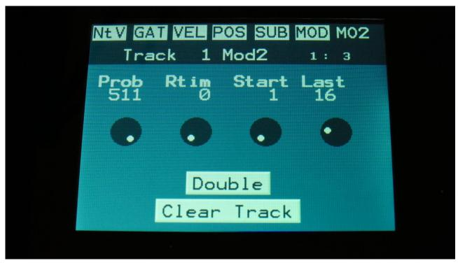
Here you can set up the track Note Randomizer, the start step and the last step of the track. It is also possible to clear or double the track.
