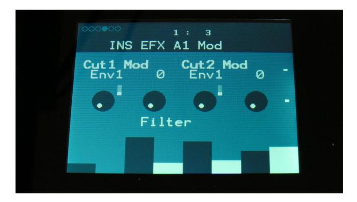
**Cut1 Mod:** Select a modulation source and adjust the amount of modulation for the Cut parameter. The small VU-meter next to the modulation source selector, shows the output of the selected modulation source.
