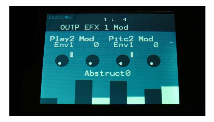
**Play2 Mod:** Select a modulation source and adjust the amount of modulation for the Play2 parameter. The small VU-meter next to the modulation source selector, shows the output of the selected modulation source.
