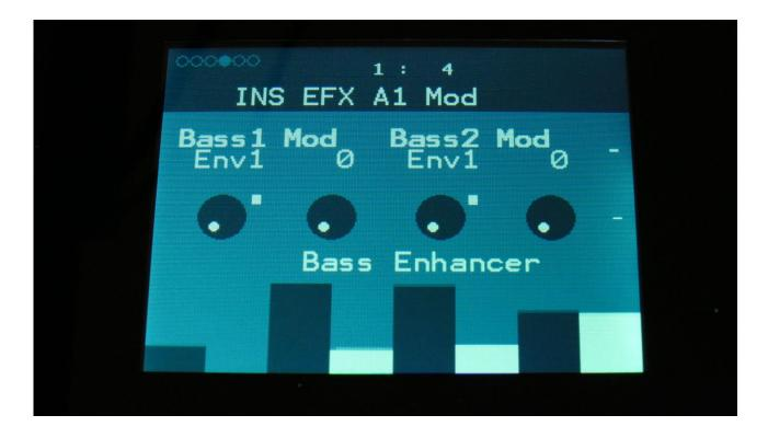
**Bass1 Mod:** Select a modulation source and adjust the amount of modulation for the Bass parameter. The small VU-meter next to the modulation source selector, shows the output of the selected modulation source.
