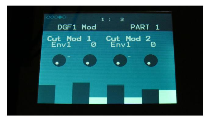
**Cut Mod 1, Cut Mod 2:** Select a modulation source and adjust the amount of modulation for the Cut parameter. The small VU-meter next to the modulation source selector, shows the output of the selected modulation source.
