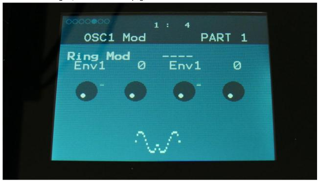
**Ring Mod:** Select a modulation source and adjust the amount of modulation for the Ring parameter. The small VU-meter next to the modulation source selector, shows the output of the selected modulation source.
