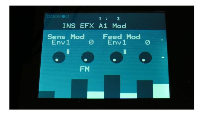
**Sens Mod:** Select a modulation source and adjust the amount of modulation for the Sens parameter. The small VU-meter next to the modulation source selector, shows the output of the selected modulation source.
