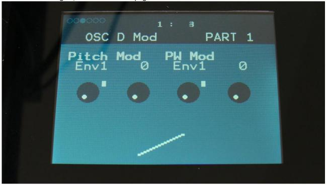
**Pitch Mod:** Select a modulation source and adjust the amount of Oscillator D pitch modulation. The small VU-meter next to the modulation source selector, shows the output of the selected modulation source.
