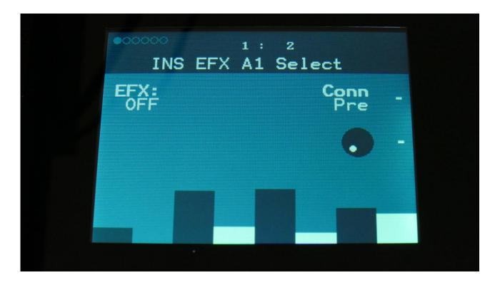
The insert effect is switched off. There are no parameters to adjust.
