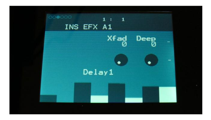
**Xfade:** Crossfade. Makes the delay effect sound smoother, by crossfading the feedback repeats into each other.
