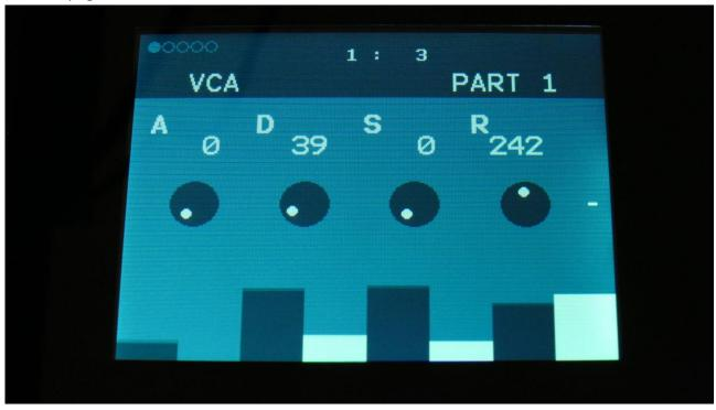
The VU-meter at the right of the screen, shows the VCA output activity.
