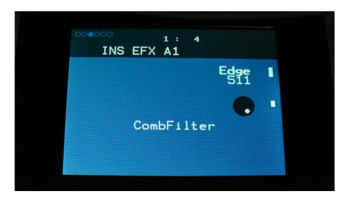
Edge: Amount of edge distortion added to the comb filter.
