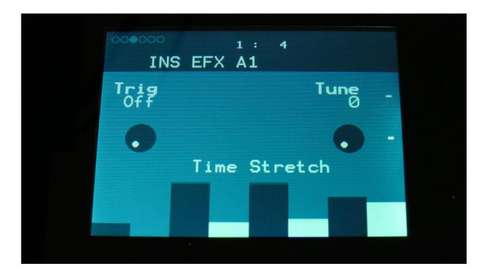
**Trig:** Off, 1 to 16. Determines if the time stretch effect should be trigged by a part or not.
