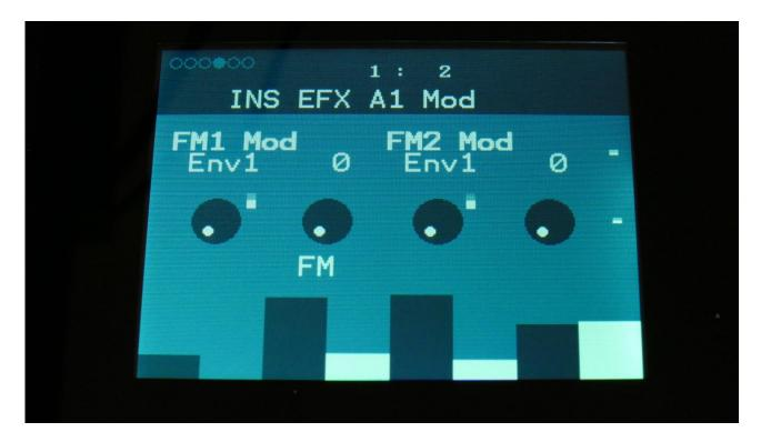
**FM1 Mod:** Select a modulation source and adjust the amount of modulation for the FM parameter. The small VU-meter next to the modulation source selector, shows the output of the selected modulation source.
