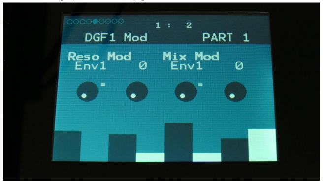
**Reso Mod:** Select a modulation source and adjust the amount of modulation for the DGF1 Reso parameter. The small VU-meter next to the modulation source selector, shows the output of the selected modulation source.
