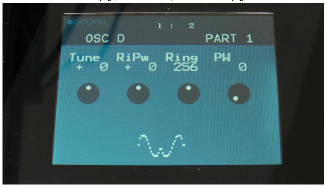
Tune: Value -64 to +63. Tunes the noise wave up and down.
