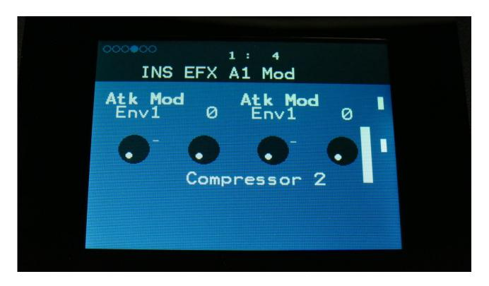
**Atk Mod:** Select a modulation source and adjust the amount of modulation for the Atk parameter. The small VU-meter next to the modulation source selector, shows the output of the selected modulation source.
