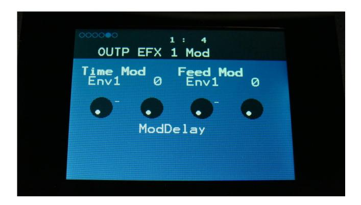
**Time Mod:** Select a modulation source and adjust the amount of modulation for the Time parameter. The small VU-meter next to the modulation source selector, shows the output of the selected modulation source.
