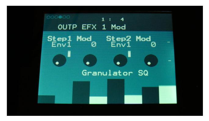
**Step1 Mod:** Select a modulation source and adjust the amount of modulation for the Step parameter. The small VU-meter next to the modulation source selector, shows the output of the selected modulation source.
