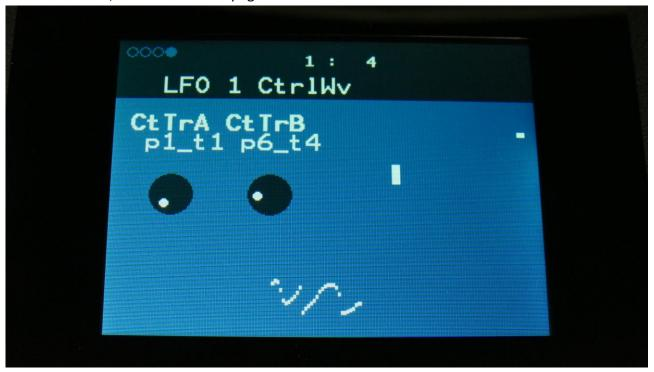
**CtTrA**: When this is set to **Off**, the LFO is running as a normal LFO, generating the same waveforms as it did before this update. When it is set to a Knob Track number (**p1\_t1** (part 1, knob track 1), **p1\_t2** (part 1, knob track 2)....**P16t4** (part 16, knob track4)), the LFO will use the values from the selected knob track to generate its waveform, when the **Wave** parameter is turned fully down, and the **Curve** parameter is set to its middle position (256).
