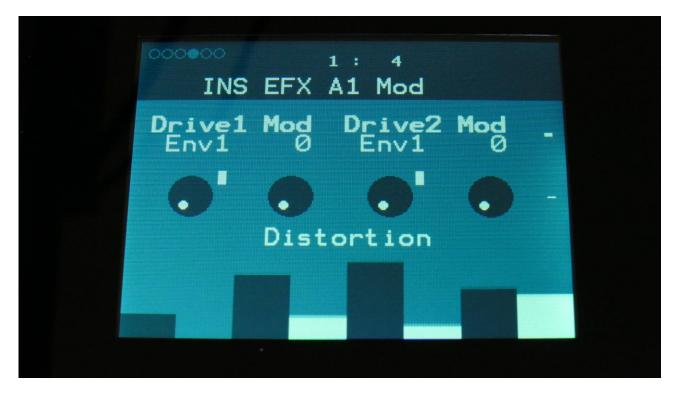
**Drive1 Mod:** Select a modulation source and adjust the amount of modulation for the Drive parameter. The small VU-meter next to the modulation source selector, shows the output of the selected modulation source.
