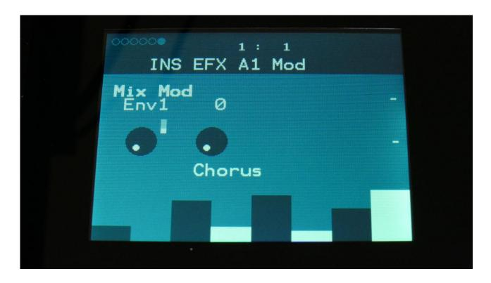
**Mix Mod:** Select a modulation source and adjust the amount of modulation for the Mix parameter. The small VU-meter next to the modulation source selector, shows the output of the selected modulation source.
