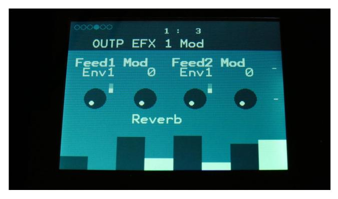
**Feed1 Mod:** Select a modulation source and adjust the amount of modulation for the Feed parameter. The small VU-meter next to the modulation source selector, shows the output of the selected modulation source.
