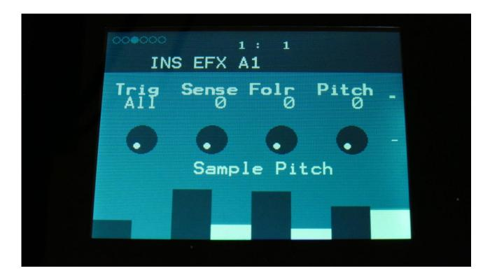
**Trig:** Off, 1 to 16, OffM, 1M to 16M. Determines if the sample pitch effect should be trigged by all parts or a single part. The "M" suffix indicates that the playback pointer will be moving in another pattern, that will give slightly different results.
