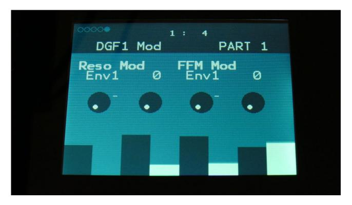
**Reso Mod:** Select a modulation source and adjust the amount of modulation for the Reso parameter. The small VU-meter next to the modulation source selector, shows the output of the selected modulation source.
