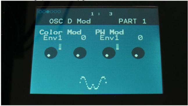
**Color Mod:** Select a modulation source and adjust the amount of modulation for the Color parameter. The small VU-meter next to the modulation source selector, shows the output of the selected modulation source.
