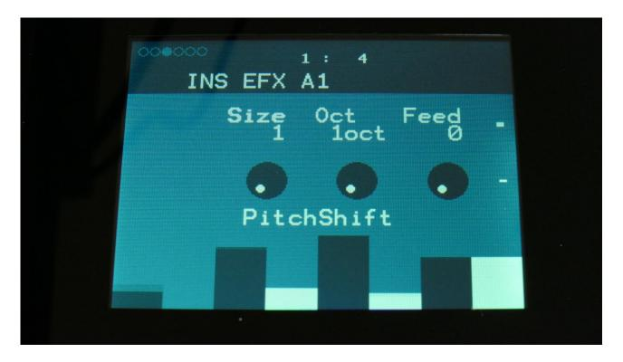
**Size:** 1 to 64. This sets the size of the buffer, used for the pitch shifting effect. When pitch shifting more complex sounds, it might make the pitch shifting more precise, when turning this parameter up a bit.
