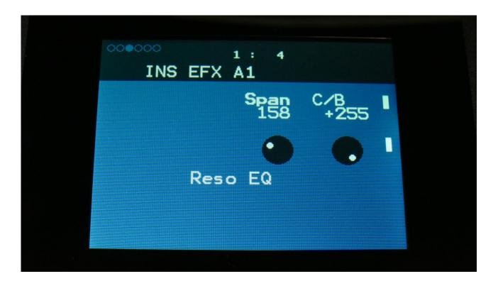
**Span:** Sets the width of the frequency band, which will be cutted/boosted.
