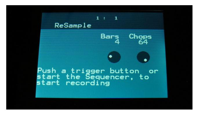
To start the Resampling, start the sequencer, or hit any of the 16 trigger buttons. Sample recording will now start:
