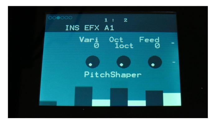
**Vari:** Pitch variation. The more this is turned up, the more the pitch variations on the input signal affects the pitch shaper frequency.
