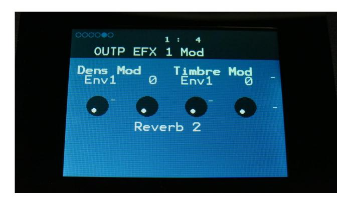
**Dens Mod:** Select a modulation source and adjust the amount of modulation for the Dens parameter. The small VU-meter next to the modulation source selector, shows the output of the selected modulation source.
