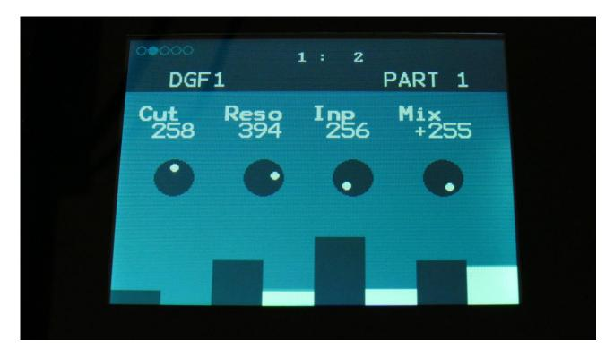
**Cut:** 0 to 511. Sets the cutoff frequency of all 3 filters at the same time. To offset the cutoff's, adjust the Spaze parameter, explained on the next page.
