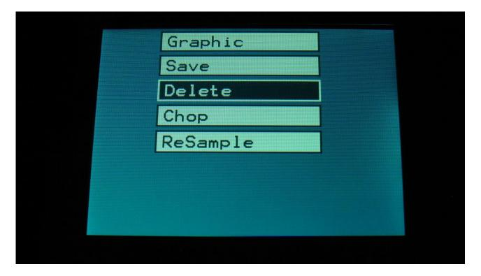
Navigate to Delete, using the < and > buttons, and then hit the Edit button, or touch the Delete module on SpazeDrum Black.
