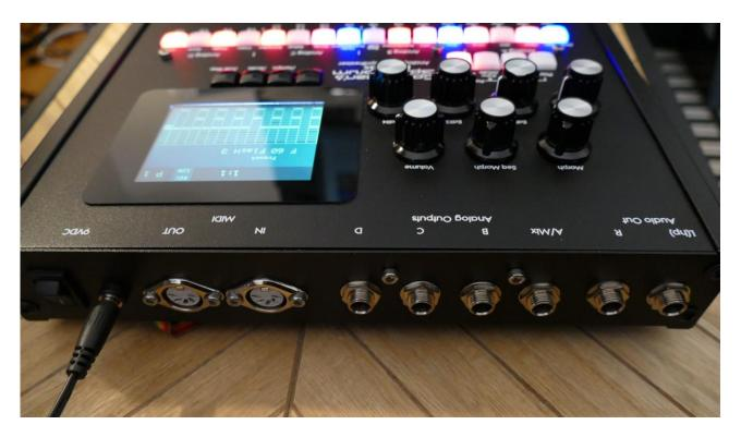
On the back panel of your SpazeDrum, you will find the power switch, connection for power supply, audio outputs and MIDI in and out.
