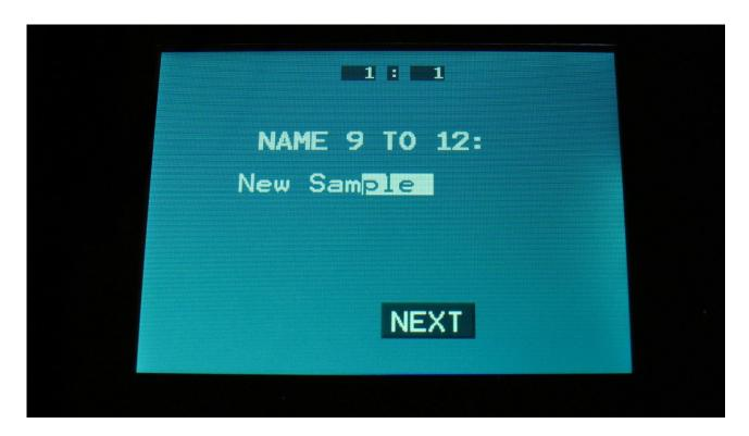
Input the next 4 characters of the name for the new sampling, using Edit Knob 1 to 4.
