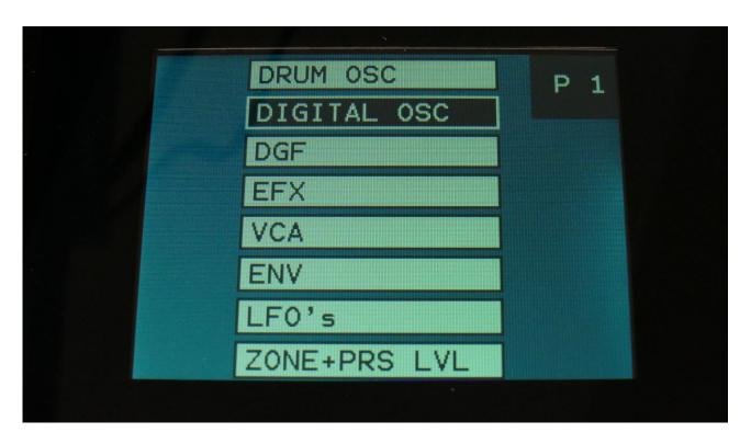
To enter the digital oscillator, select DIGITAL OSC by using the < and > buttons, and then push the Edit button.
