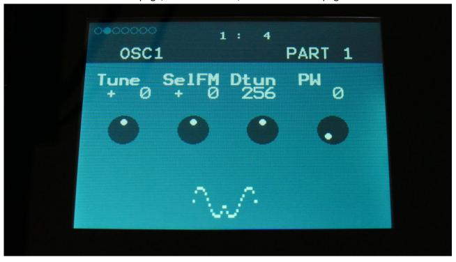
**Tune:** Adjust the basic pitch in semitones. Range: -64 to + 63.
