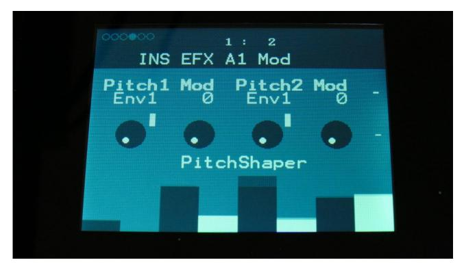
**Pitch1 Mod:** Select a modulation source and adjust the amount of modulation for the Pitc parameter. The small VU-meter next to the modulation source selector, shows the output of the selected modulation source.
