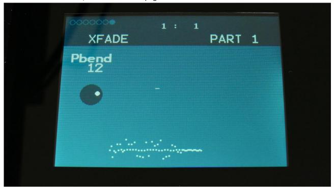
**Pbend:** Sets the pitch bend range for the part in semitones. Off, 1 to 12.
