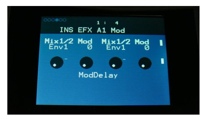
**Mix1/2 Mod:** Select a modulation source and adjust the amount of modulation for the Mix1/2 parameter. The small VU-meter next to the modulation source selector, shows the output of the selected modulation source.
