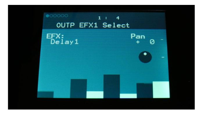
The 2 VU-meters at the right of the screen, shows the Effect input and output activity.
