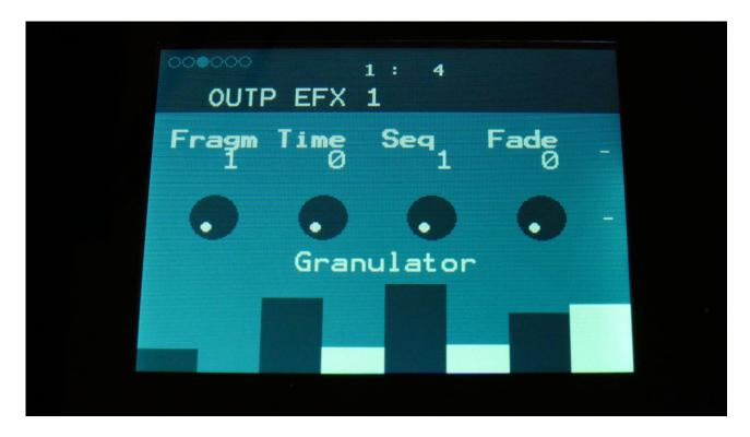
**Fragm:** Sets how many fragments (or grains) the input signal should be cutted up in. Possible values are 1, 2, 4, 8, 16, 32, 64 or 128.
