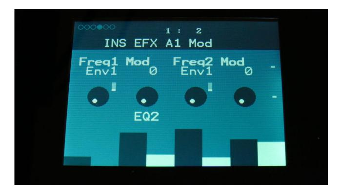
**Freq1 Mod:** Select a modulation source and adjust the amount of modulation for the Freq parameter. The small VU-meter next to the modulation source selector, shows the output of the selected modulation source.
