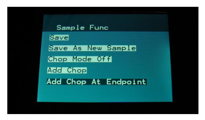
Select "Add Chop At Endpoint", using the < and > buttons, and push the Edit button. SpazeDrum will now jump back to the graphical sample edit page, and a chop point will be added at the selected end point.
