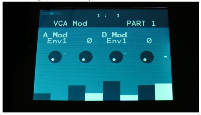
**A Mod:** Select a modulation source and adjust the amount of modulation for the Attack parameter. The small VU-meter next to the modulation source selector, shows the output of the selected modulation source.
