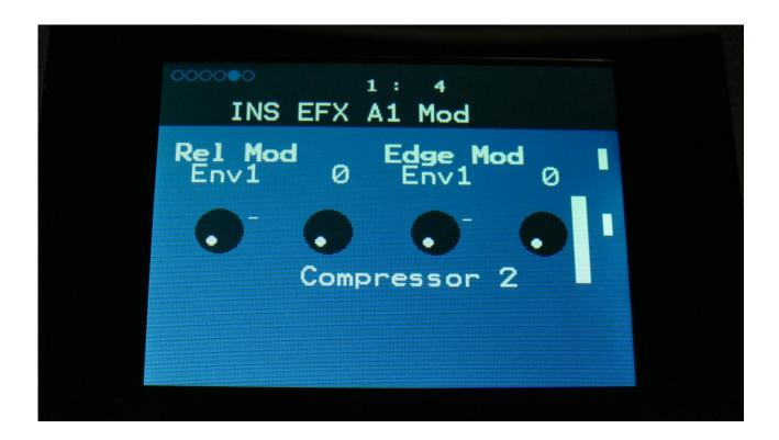
**Rel Mod:** Select a modulation source and adjust the amount of modulation for the Rel parameter. The small VU-meter next to the modulation source selector, shows the output of the selected modulation source.
