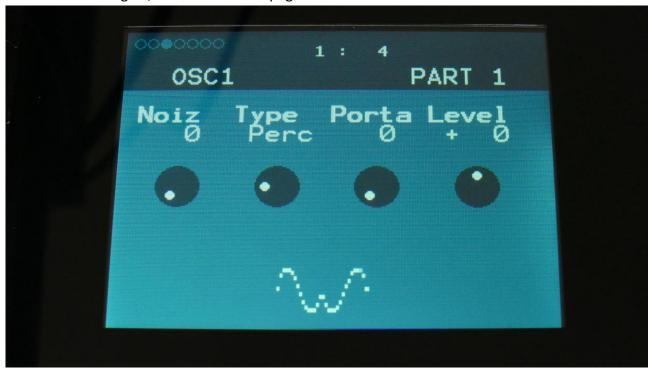
Noiz: Adds noise FM to modulate the pitch of the percussion waves. Range: 0 to 511.
