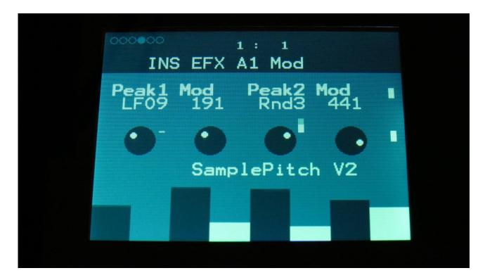
**Peak1 Mod:** Select a modulation source and adjust the amount of modulation for the Peak (formant) parameter. The small VU-meter next to the modulation source selector, shows the output of the selected modulation source.
