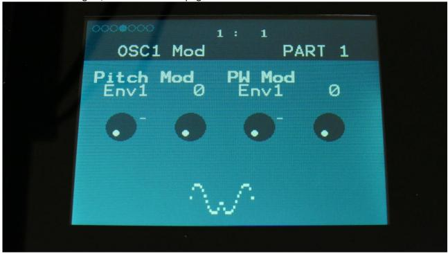
**Pitch Mod:** Select a modulation source and adjust the amount of pitch modulation. The small VU-meter next to the modulation source selector, shows the output of the selected modulation source.
