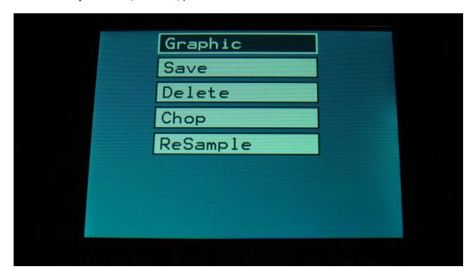
Navigate to Save, using the > button, and press the Edit button, or touch the Save module on SpazeDrum Black. The display will now show "Saving Sample..." for a short while, and return to the main sample edit page.
