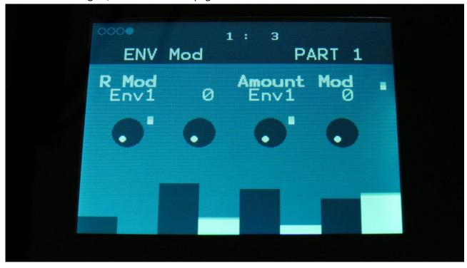
**R Mod:** Select a modulation source and adjust the amount of modulation for the Release parameter. The small VU-meter next to the modulation source selector, shows the output of the selected modulation source.
