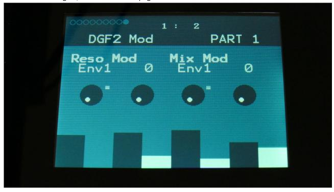
**Reso Mod:** Select a modulation source and adjust the amount of modulation for the DGF2 Reso parameter. The small VU-meter next to the modulation source selector, shows the output of the selected modulation source.
