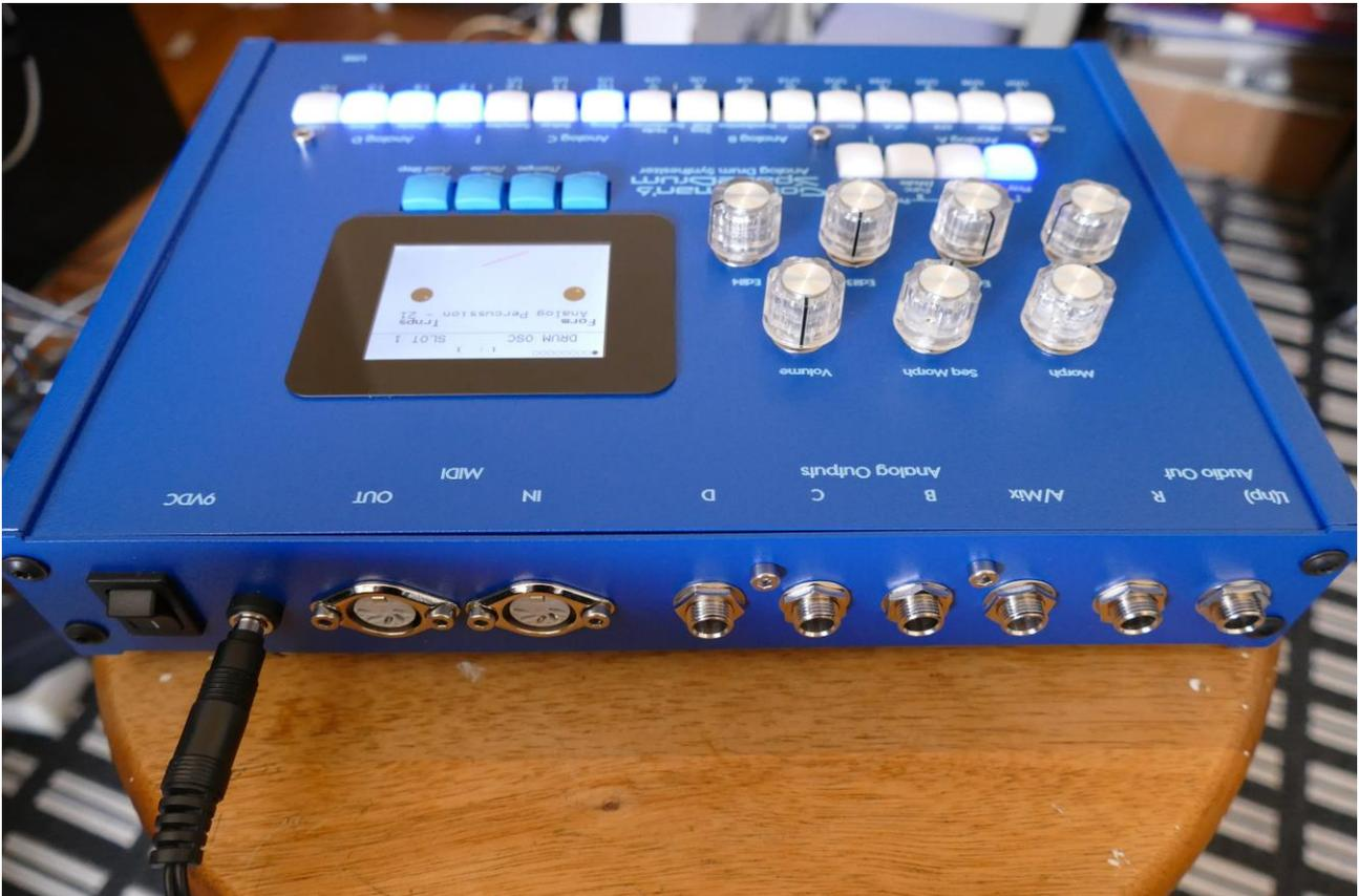
On the back panel of your SpazeDrum, you will find the power switch, connection for power supply, audio outputs and MIDI in and out.
