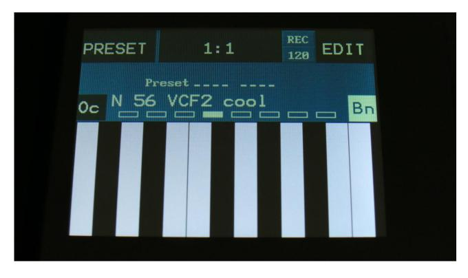
In this firmware version, the "old" touch screen keyboard with a lot of tiny keys is gone. Now the keyboard will always be one octave wide, to have the touch keys as large as possible.
