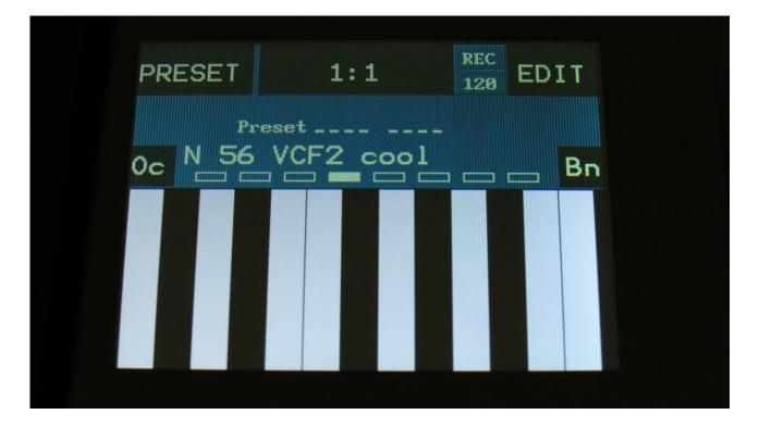
When the keyboard is not in bend mode, swiping your finger over the it, will make it trigger each note.
