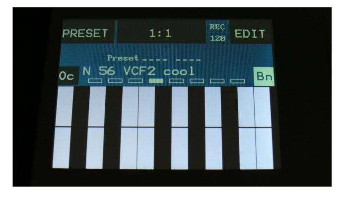
When 2 octaves are selected, the upper and lower octaves get divided by a line in the middle of the keyboard. When 3 octaves are selected, the upper, middle and lower octaves get divided by 2 lines.
