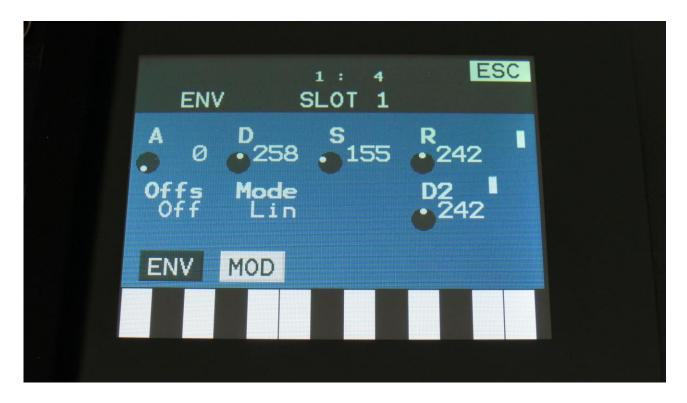
An output VU-meter has now been added to the Decay Envelope, near the D2 parameter.
