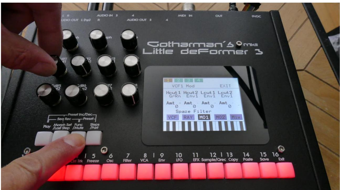
To select a specific modulation source, within the selected group, simply push and hold the Steps/Part button, while turning one of the modulation source select parameters. Again, you can release the Steps/Part button, as soon as you have turned one of the parameters, and select the modulation source for each parameter. LD3 will stay in this mode, until you go back to select a group, or until another edit page is selected.
