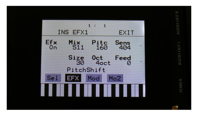
A Size parameter has been added to the PitchShifter effect. This sets the size of the buffer, used for the pitch shifting effect. When pitch shifting more complex sounds, it might make the pitch shifting more precise, when turning this parameter up a bit. Range: 1 to 64.
