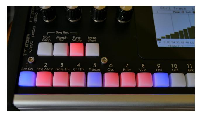
When you are located on a sequencer controller track, and selects the button Bar Select function, it is now possible to access all 8 bars of a controller track via the push buttons. Step button 2 to 9 equals Bar 1 to 8. The button of the bar that is selected will light up, the other 7 buttons will flash.
