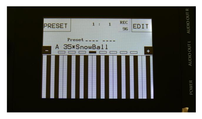
When parameter changes has been made to a preset, and these changes has not been saved, a "\*" will now appear, right between the preset number and the preset name, on the main Preset Select page.
