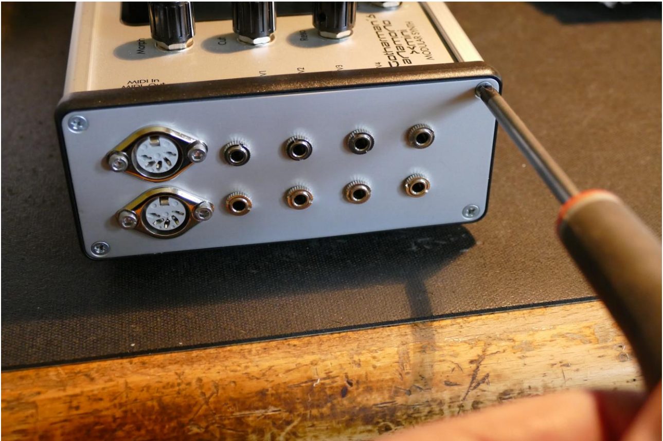
Remove the 4 screws in the corners of the left endplate, using the Phillips screwdriver.
